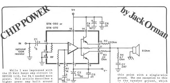
either the Sanyo STK-050 (50 Watts) or STK-070 (70 Watts). How it works. Figure 1 is an
