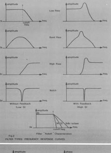
back). You can see that feedback around a filter creates a "peak" at the cutoff frequency of the filter.
