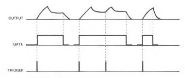
FIG.2 TIMING DIAGRAM / DUAL ADSR
