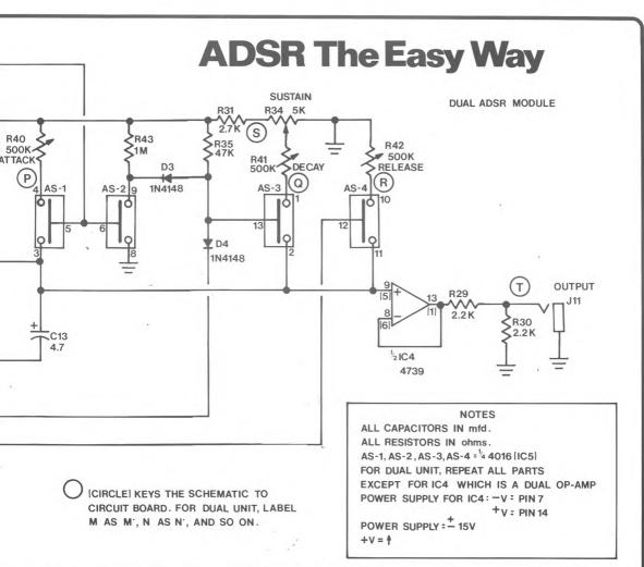
the voltage present on C13; when this voltage reaches +10V, the flip-flop in the 555 shuts off, which brings pin 3 low and opens AS-1. This ends the attack portion of the cycle.
