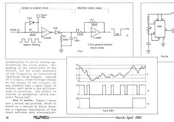
half the supply voltage, you can get false triggering as shown in figure 3. However, if we apply some hysteresis around a buffer, then the circuit acquires more noise immunity since the buffer now has two trip points. The voltage must drop below about 1.3V to turn the touch switch off, but rise above 4.2V to turn it back on. No matter what happens in between these two points, the switch will remain stable.
