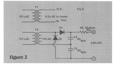
technique used in many inexpensive television sets, and when used around audio equipment is a good way to get 117V flowing through your body. Always (repeat, ALWAYS) use an isolation transformer; it's not expensive considering the safety factor it provides.
