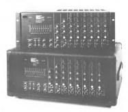
Programmable EQ. The PEQ-1 from Polyfusion (92 Benbro Drive, Buffalo, NY 14225) is a 16 band programmable EQ which can store up to 64 response curves. It also includes bypass switch, balanced/-unbalanced inputs/outputs, two computer I/O ports, and more. List price is \$1,495.
