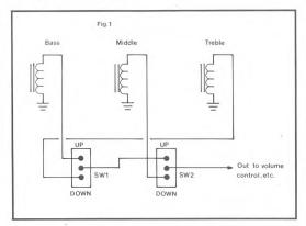
Referring to figure 1, SW1 works just like a two pickup Les Paul switch, and sends the signal from either or both pickups to SW2. SW2 selects middle pickup only, SW1 signal only, or middle pickup plus whatever SW1 is set for. I think that Gibson players can "relate" to three pickups better with this particular switching scheme. Here's an overview of the switch positions.
