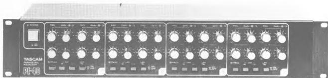
**New EQs.** Teac (7733 Telegraph Road, Montebello, CA 90640) has introduced the PE-40 four channel, four band per channel parametric EQ. In addition to the parametric EQ, each channel has three pushbutton selectable filters (two high pass and one low pass) along with a bypass switch. Claimed specs are 83 dB S/N with under 0.15% THD.
