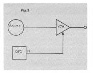
volume control. Its main benefit is that making fast level changes by touch is far superior to making volume changes with a pot. This method may process any program material in which the musical transient is already shaped. One application is processing prerecorded tapes during mixdown to compensate for a static quality in the original program material. Tapping the sensor in time with the music creates subtle, or dramatic, dynamic alterations.
