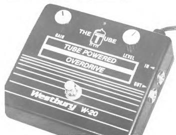
**Tube Fuzz.** Unicord (89 Frost St., Westbury, NY 11590) has announced The "Tube", an overdrive circuit based on a 12AX7 tube instead of solid state circuitry.
