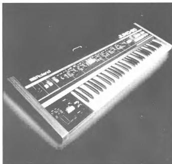
The JUNO-60 is a programmable poly synth with 5 octave keyboard, 56 programs organized as 7 banks of 8 programs, arpeggiator, transposer, chorus, etc. There's also a Digital Communication Bus designed to interface to the Roland MC-4 microcomposer, digital sequencers, and similar devices for programmed performances. \$1795 list.
