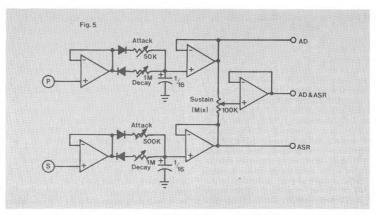
this circuit, the dynamic range control is reduced to a single pot. At one extreme, it offers the full dynamic range; rotating the control gradually compresses the dynamic range until at the other extreme of rotation, the output is a static waveform.
