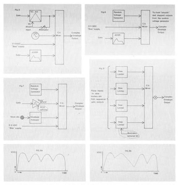
input. Other spacings produce quite a variety of envelopes; figure 8c is an example of an "irregular" envelope. The amount of slew limiting should be adjusted to taste.
