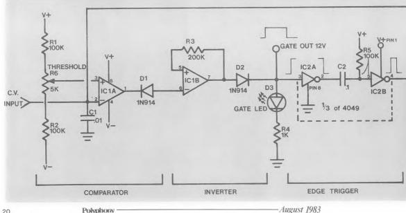
ents and the voltage will swing all the way to +15V, however PAIA EK-x circuits handle a 12V gate voltage just fine as is.
