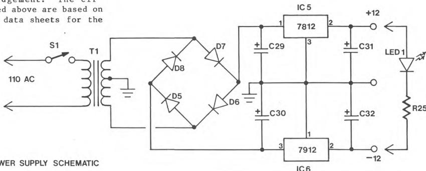
FIG. 4 POWER SUPPLY SCHEMATIC
