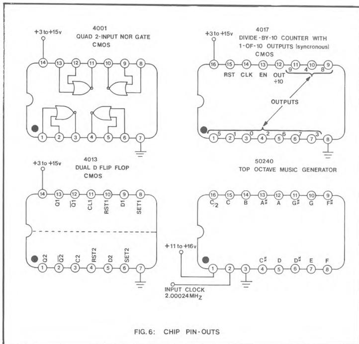
FIG. 6: CHIP PIN-OUTS
