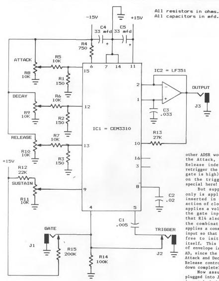
C2 is not a timing capacitor, but instead compensates an amplifier internal to the CEM3310. Likewise, resistor R4 has nothing to do with the time constant, but is instead a dropping resistor for the internal Zener diode. A value of 750 ohms is recommended for safe operation with a  $\pm 15V$  supply.
