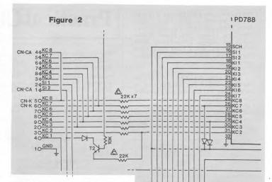
Octave drops. Another option is software octave drop; while different preset sounds use this function, it is not normally accessible so that you can octave drop any sound. To make this possible, add a switch and diode in series between LSI pin 25 (KC8) and pin 16 (SI-1; see Figure 3).
