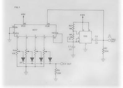
The circuits. Figure 1 shows a four-stage model that uses only two ICs, and could easily be expanded to 10 stages with the addition of a few more pots and diodes. Of course, it is missing a few features which would make it easier to set up and adjust, but for a simple starting point it works just fine.
