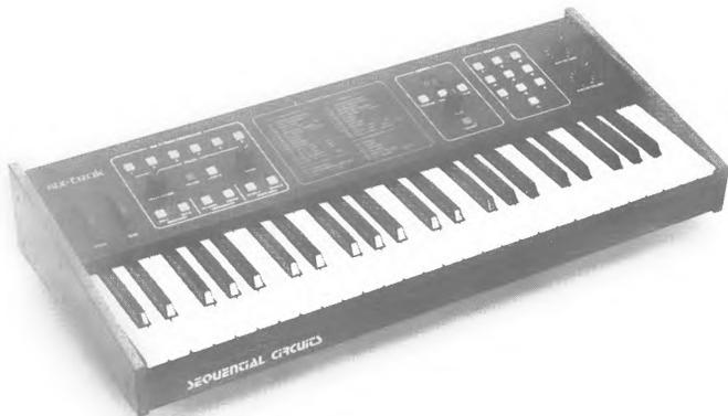
The Sequential Circuits Six-Trak synth is a polyphonic keyboard with the unique ability to store two multi-timbre real-time sequences of six different tracks; total on-board memory is 800 notes. The Six-Trak also expands to over 4000 note memory when used with a Commodore 64 and Sequential's own "Sequencer 64" module. In fact, SCI's compositional package, which includes their "Drumtraks" as well, gives the user more songwriting power than ever available before in so reasonably priced a system.
