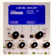
Synchrosonic™ measures the audio delay between the main and fill speakers, then automatically sets the time delay necessary to make the audio synchronous—eliminating delay and phasing problems
