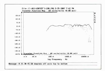
a large room on a 6 foot stand. Using time windows then gives equivalent anechoic results above 200 Hz including front panel reflections and cabinet diffraction; overall results give true acoustical summation of all drivers and passive radiating elements.
