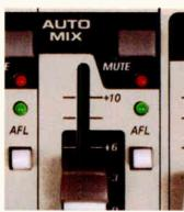
Automix™ is an 8-channel gain-sharing protocol that tames the comb filtering and phasing issues that occur when multiple microphones compete for dominance in the mix
