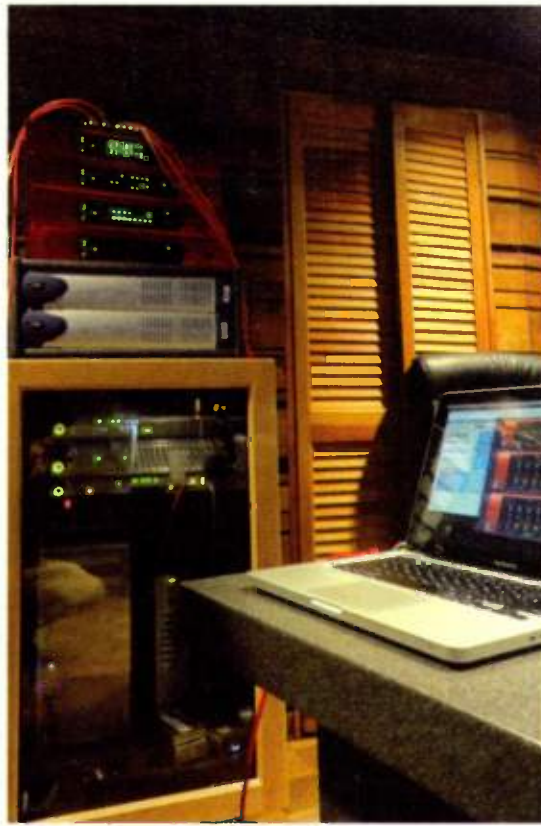
Focusrite Rednet Modules atop an Omega Studios gear rack, with RedNet control running on the laptop in the foreground.
