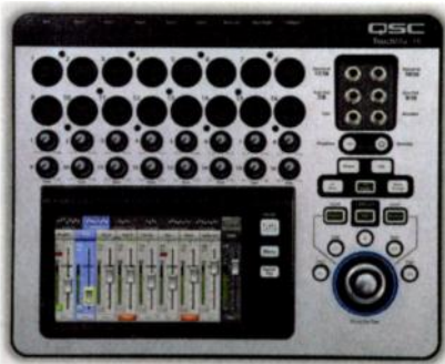
QSC's TouchMix-16 combines an embedded touchscreen mixer with key buttons and faders.
