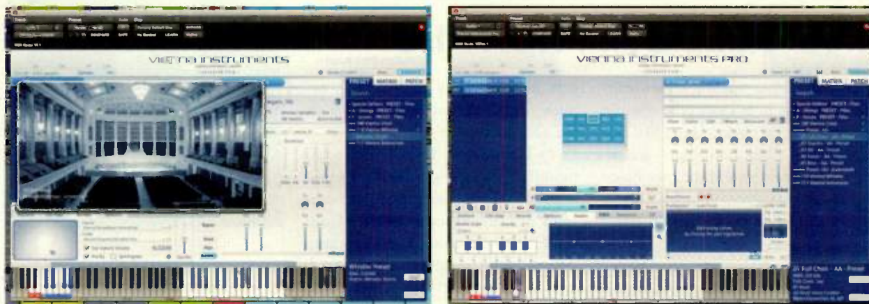
Left: MIR Pro Venue is a multi-impulse convolution application with purchasable RoomPacks featuring world-class concert halls, scoring stages, churches and more. Right: Comprehensive parameter displays are shown in the Advanced View window.
