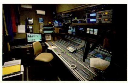
A Calrec Apollo digital audio console was the centerpiece in the Game Creek Video production truck used for the US Open—one of seven Calrec consoles deployed for the Fox Sports coverage
