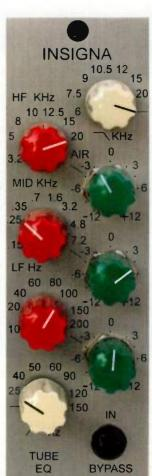
The INSIGNA is a tube EQ for the 500 Series format featuring rich second harmonic triode tube colorization.
