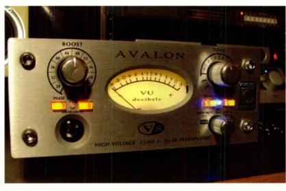
The Avalon V5 half-rack width DI and mic preamplifier.
