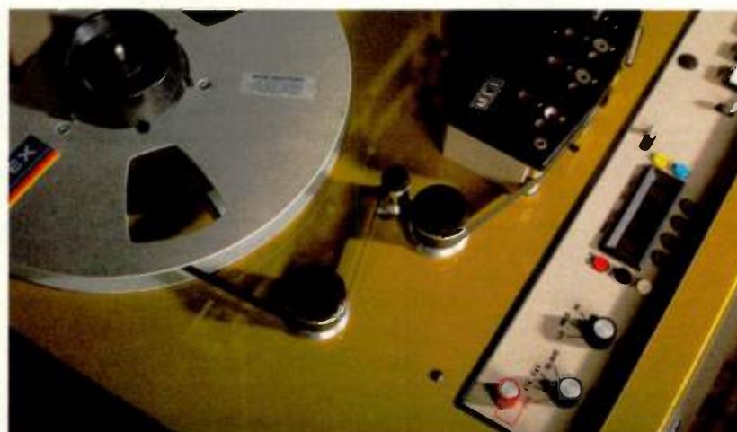
The recorder stores alignments for all speeds and makes it easy to toggle between 7.5, 15 and 30 IPS so the user can compare the differences before committing to a favorite speed.
