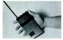
Figure 12. An integrating and computing handheld SLM.
