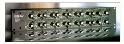
based around the 4558 op-amp chip for each of the parametric sections. The same op-amp is used for the shelving filters and for the electronic input balancing. All the circuitry is run from 18V rather than the more usual 15V, presumably to make the best use of the available headroom, and the general standard of design is up to the quality you'd expect from Ashly.
