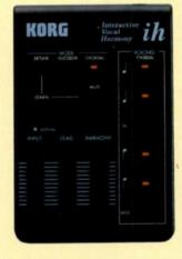
work with any MIDI keyboard, but ideally suited to work in tandem with an i-series keyboard, the ih offers three different effect modes — Chordal, Vocoder and Detune. A maximum of four harmony notes can be generated to match a chord input from a MIDI device, or in response to SysEx messages from an i-series keyboard; Detune offers a subtle detuning effect to thicken or enrich the input signal.
