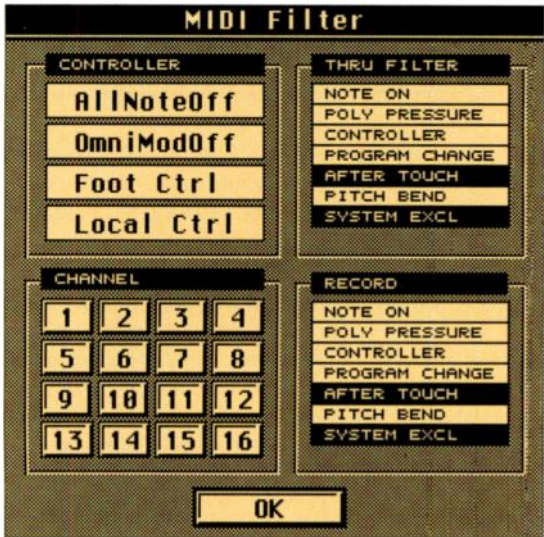
Figure 3: Cubase's MIDI Filter box.
