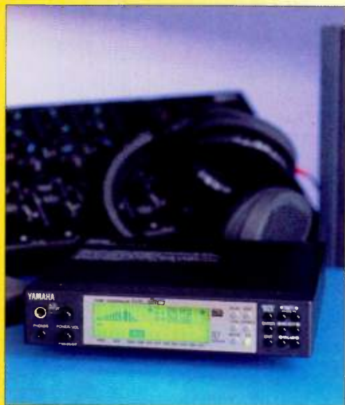
External MIDI modules like the Yamaha MU50 that can connect directly into the PC's serial port can give the best of both worlds.
