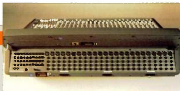
The rear view. Most of the connectors are quarter-inch jacks, apart from the XLR mic inputs.
