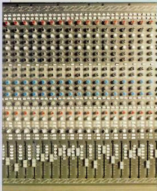
The Topaz Project 8's in-line channel strips in close-up.
