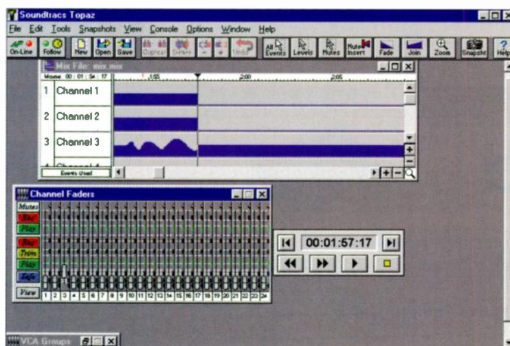
The automation software showing all of the channels on the 24-channel Project 8. Above this are the graphical representations of the fader data for the first four channels.
