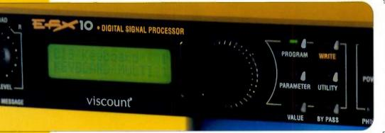
editor in a sequencer program like *Cubase*. Usefully, you can dump the EFX10's whole memory (or just parts of it) to a suitable storage device or computer over MIDI; bulk dumping is initiated in Utility mode.
