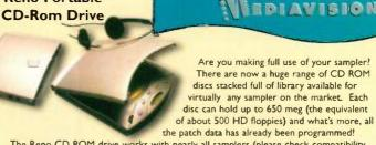
The Reno CD ROM drive works with nearly all samplers (please check compatibility when ordering) as well as Mac and PC. Most CD ROM drives can play audio CD's, but require special software on a computer to do so. The Reno though has integral buttons for playback and track search etc, and can even be run off batteries for use as a portable CD player (headphones included). We have managed to secure a quantity of these at a huge discount - order now whilst stocks last!
