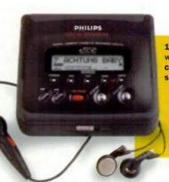
18 bit portable recorder with digital i/O, where dremote, analogue cassette compatibility and stereo mic. input-sonically identical to DCC730/951.
