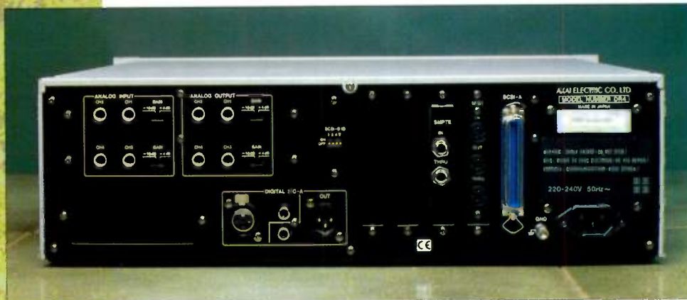
The DR4vr's well-furnished back panel, including digital In and Out in both SP/DIF and AES/EBU formats. Two more channels of digital I/O can be added with an optional board.
