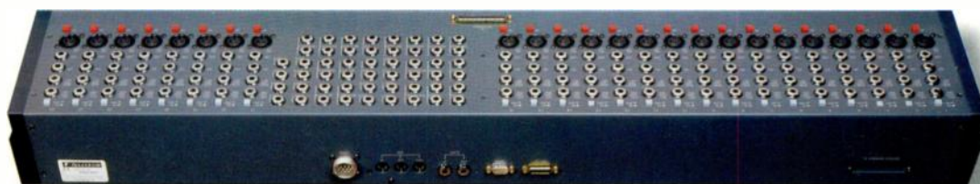
The Ghost's connectors and back panel, including MIDI sockets.
