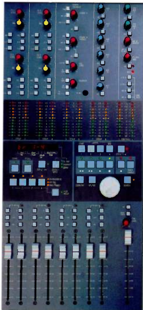
The Ghost's Foldback and Aux Return level controls, MMC control panel, and Group faders.
