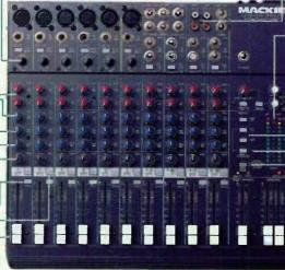
All inputs & outputs are balanced to out A hum & allow extralong cable runs, but can also be used with unbalanced electronics. <sup>1</sup> except RCA tape jacks, heaphone jack & inserts
