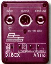
BSS's fully-featured AR116 active DI box offers a low-pass filter, a choice of three types of pad (for use with guitar pickups, line-level inputs, and power amp speaker outputs), a ground lift switch to help prevent earth loops, and an XLR output.
