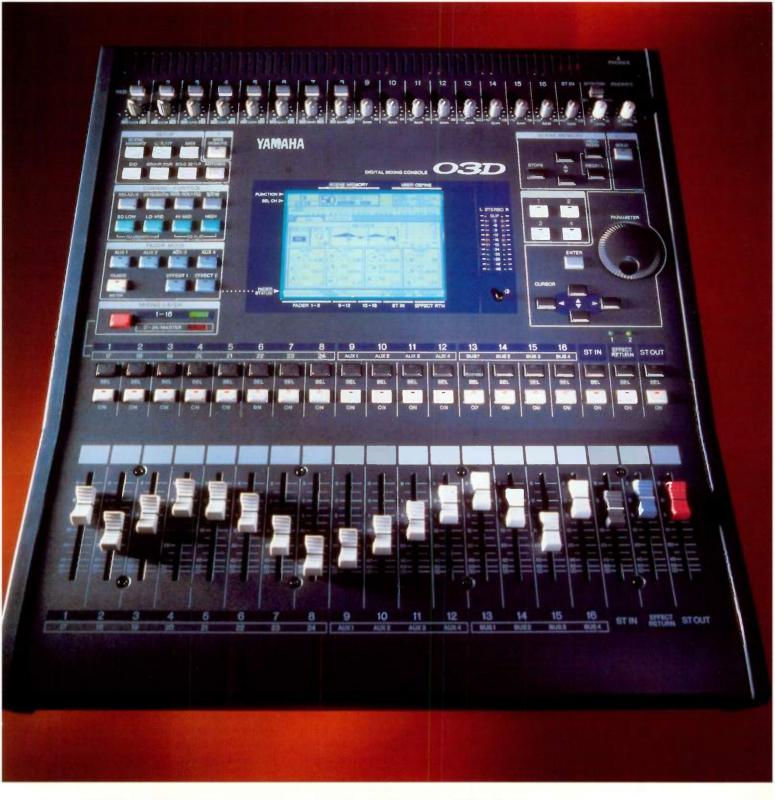
boxes, with all the related operations gathered together. At the top, eight white push buttons are grouped under the heading of 'Setup'. These are used to configure the basic operation of the desk, giving access to the Scene Memory stores, various utilities (a line-up oscillator, user preferences, and so on), MIDI functions, digital I/O facilities (including dithering options), channel and fader grouping or pairing, solo monitoring modes, and Automix setup and editing operations (see below).
