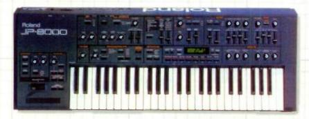
Analog Modelling not only produces superb emulations of the great synths of the 60's and 70's, but also totally unique timbres never before heard. Realtime control is excellent, and all knobs, sliders, buttons and the ribbon controller send out Continuous Controller messages. For instant creativity, a powerful arpeggiator and real time phrase synthesiser are included, which can be easily synchronised to an external MIDI clock. This is very likely to be the hottest synth of '97 - order now!
