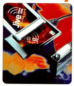
otebook PC users looking for a General MIDI/Wavetable card now have another option in the £129.95 Jive WaveTable from Chase Advanced Technologies. This PCMCIA card, which is also equipped with a joystick controller, provides 128 GM-compatible instruments plus 61 drum sounds, and even offers an FM synth for use with older games that don't support wavetable cards.
