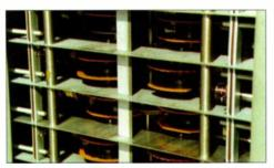
A very rare picture of the tonewheels. The edges are painted orange to prevent corrosion.
