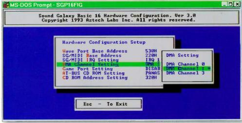
Figure 4: Here is a simple DOS application, in this case a utility for setting up an old soundcard, running inside a window under Windows 95. The blocky graphics may look primitive, but the entire screen display will only take up 1000 bytes of memory when running in its native full-screen DOS mode!
