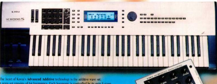
The heart of Kawai's **Advanced Additive** technology is the additive wave set. A wave set consists of 64 harmonics. Each harmonic is controlled by its own 5 stage, cooping amplitude envelope. The 128 band Formant Filter can simulate natural tonal characteristics, and 123 PCM samples such as classic analogue synth waveforms addextra spice. Up to 6 elements can be combined to create amazing complex timbres.
