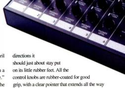
Each of the six channels has an overall level control at the bottom (for the main stereo mix), four individual controls to add the four mono inputs (A, B, C, and D), and an effects return level. On the back panel, the headphone outputs are on standard stereo jack sockets, as you'd expect. Beneath these are the effects
