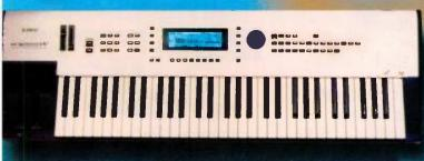
(5000 Workstation adds General MIDI Synthesis with 341 waveforms and 225 rum waves to the additive section giving 64 note Polyphony. Also includes a lowerful 50,000 note, 40 track sequencer with 32 MIDI channel support.
