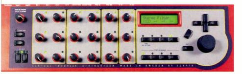
The Nord Modular's hardware front panel, with its 18 freely assignable knobs. The four Patch Group buttons for selecting the Slots are at the bottom right.
