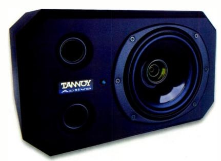
The 165mm (6.5-inch) bass-mid cone is supported by a nitrile-rubber surround on the outside edge, with an inner suspension arranged to allow the cone to slide up and down on the outer of the three brass tubes. The user manual proudly professes that the motor system (ie. the magnet and voice-coil assembly) has been "computer optimised" in terms of coil-winding parameters and magnetic flux strength in the air gap.
