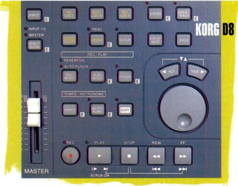
► It's also possible to apply stereo effects to the whole mix, or even to monitor via the effects while recording, without recording the effects. Setting up these various options necessitates a little menu cruising but it's something you'd soon get used to.
