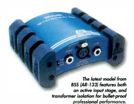
to match a guitar to a mixing desk, the output side of the transformer is required to deliver a higher current than the original signal source, which means a significant drop in signal voltage. To overcome this, the DI box needs to be be plugged into a console mic input, where sufficient gain is available to restore the signal level.
