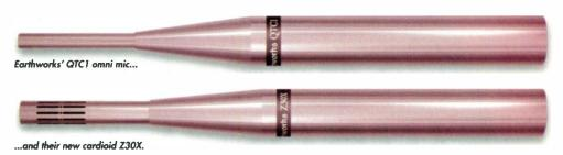
Its front pick-up pattern is like a very open cardioid, with a claimed greater rejection at 90 degrees than most directional mics. The rear half of its pickup pattern resembles a good hypercardioid. It has a high SPL of 145dB, improved noise of 22dB (A-weighted), and is intended for natural, uncoloured close-miking of most instruments and vocals.
