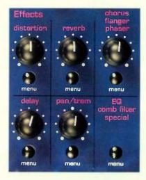
A front-panel section labelled 'effects' provides an adjustable control knob and a menu button for each of the seven effect-types.
