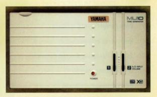
The Yamaha MU10 only has a line level input, so it's not ideal for direct recording of electric guitar.
