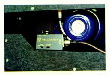
The Palmer Junction passive speaker simulator/DI will accept a speaker-level input, but does not include a dummy load.
