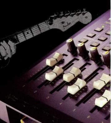
The D8's input connections accept anything from keyboards and samplers to guitars and microphones, and its S/P DIF input lets you record from DAT or CD digitally, keeping the original sound quality. The built-in sample rate converter ensures everything inside the D8 is at the CD-compatible sample rate of 44.1kHz. At mixdown, you can use the main and aux inputs to add an extra four channels.
