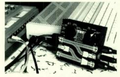
The TS1 merges MIDI data received with its own sync data. You won't need to swap around the MIDI wiring, as TS1 has four MIDI ports and automatic signal routing.
