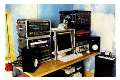
Racks in a rack, including (left rack): a Roland MPG80 Super Jupiter Programmer & MKS80 synth, Waldorf MIDI bay, Roland A110 MIDI display and M480 48input line mixer; (right rack) Studio Electronics SE1 'Minimoog in a rack', Sequential Prophet VS, Clavia Nord Rack Yamaha TX802, Emu Vintage Keys, Novation DrumStation & BassStation rack, Akai \$3000 sampler. The Novation BassStation keyboard is also visible on the right.
