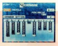
The Technics KN5000 virtual drawbar acoustic modelling, first used on the WSA synths.
