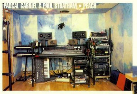
Left: The Strongroom setup. Left to right, top to bottom: ARP Odyssey & Sequential Circuits Pro One synths, Mackie 32°8 mixer, Korg Mono/Poly analogue synth (on the floor), Dynaudio monitors. In the rack on the right are the Empirical Labs compressor, the dbx 120X DS Boom Box, an Alesis D4 drum module, the Mutator Mutronics filter bank, an Oberheim Matrix 6R, and the Roland SPV355 pitch-voltage synth.
