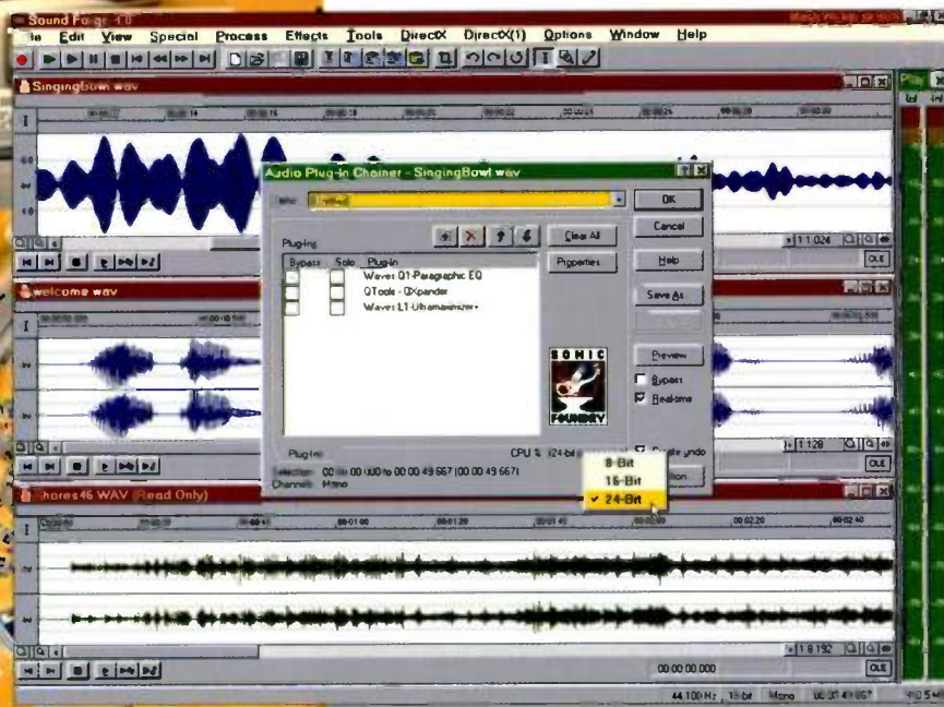
Figure 4: The Audio Plug-In Chainer of Sound Forge allows 24-bit processing to be carried out on a chain of plug-ins, without ever dropping back to the 16-bit resolution of the file itself.
