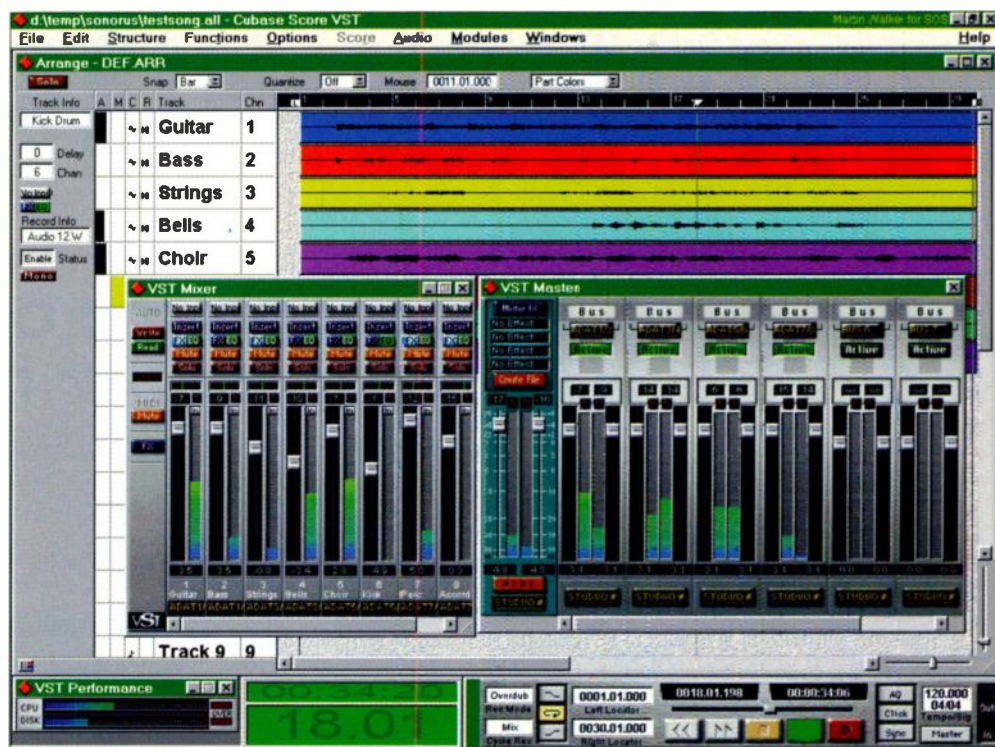
Figure 3: The Sonorus STUDI/O interfaces easily with Cubase VST. Here eight pre-recorded tracks (moved en masse from an ADAT tape) have been routed back to the STUDI/O ADAT outputs.
