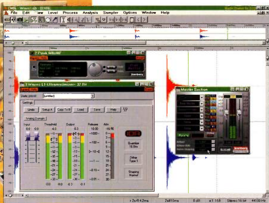
Figure 1: You can insert up to six real-time plug-ins in Wavelab 2.0, and then apply them simultaneously with 32-bit calculations. Two dynamics processors are also shown here: Peak Master is included free with Wavelab, and Waves' L1 Ultramaximizer is part of the famous Native Power Pack. Notice that both the L1 and Wavelab's Master Section currently have dithering enabled. You should choose one or the other for best results.
