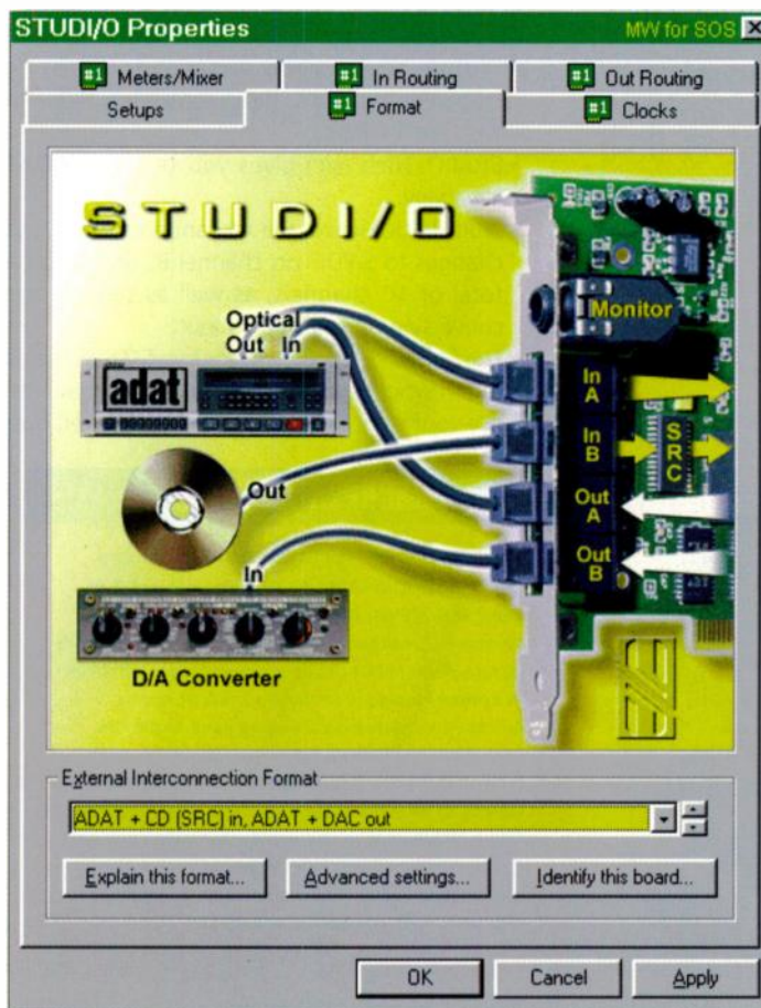
Figure 1: A host of options is provided in the Format page of Properties — many combinations of equipment are already included as presets, such as the ADAT plus CD digital inputs (10 input channels in total), and ADAT and external stereo converter (10 output channels) shown here.
