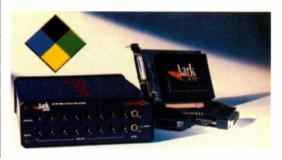
The Aark 20/20 comes complete with HOST PCI card, 10 channel AD/DA/digital i/o interface box, interface cable, control panel software and Samplitude Basic by SEK'D, multichannel audio editing CD-ROM. - That's everything you need to turn your PC into a high quality multitrack audio recording studio!
