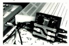
The TS1 merges MIDI data received with its own sync data. You won't need to swap around the MIDI wiring, as TS1 has four MIDI ports and automatic signal routing.
