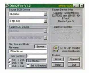
Disk2File does exactly what it says on the (virtual) tin — reads any formatted SCSI disk, and then transfers the contents to a file. Ideal for PC and sampler owners everywhere (see main text).
