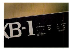
Connection to an external Leslie speaker is only possible via the the optional XLD1 Leslie adapter, which connects to this 8-pin DIN socket on the XB1's rear panel.
