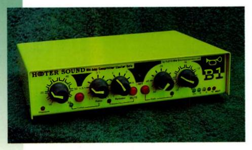
where the orange +8dB LED lights, and 2dB later, the limiter cuts in. The levels shown on the meter are accurate when the output control is set to maximum, but as many soundcards work at a reduced line input level, it may be necessary to back off the output gain. The output gain control comes after the meter.
