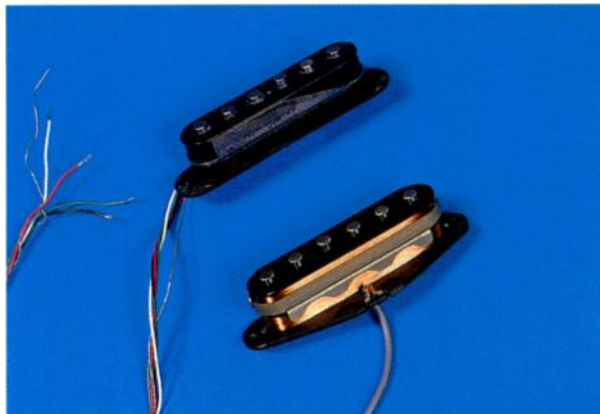
Above: Magnetic screening is used to try to minimise interaction between the coils — while DiMarzio (top) shields almost the whole of the upper coil, with a cutaway on the bass side, Kinman employs a partial shield on both, with the intriguing 'scalloped' design on the lower coil.
