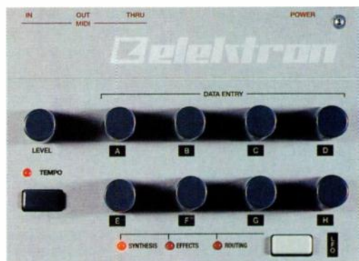
The Level control (which sets the volume of the currently selected Machine/drum sound relative to the others) and multi-purpose, MIDI-transmitting Data Entry knobs. Access to the bewildering variety of Machinedrum LFOs is also via the seemingly innocuous white button here.
