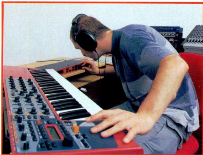
Some simple extender arms for your keyboard can make playing and editing rackmount synth modules a much more comfortable experience.
