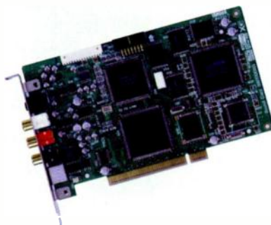
Consumer soundcards have had synths on board for a long time, but Yamaha's SW1000XG was the first soundcard to feature a professional-quality sound module built in.
