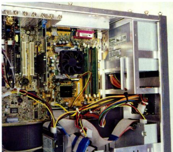
The ATI Coolermaster case is an excellent choice for the musician: its thickness provides some sound insulation, while its thermal properties mean that this PC can be run with all three chassis fans disconnected, thus generating less noise in the first place.
