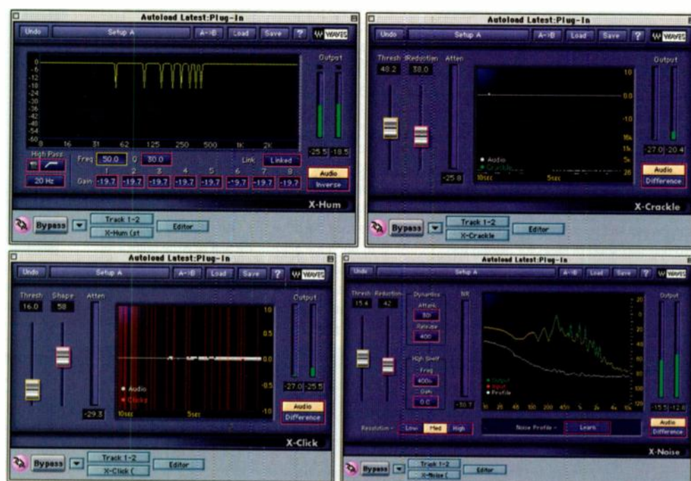
Waves Restoration Bundle, clockwise from top left: X-Hum uses a series of linked notch filters to remove fixed-frequency interference such as mains hum; X-Crackle attenuates the surface noise that can afflict old vinyl; X-Noise tackles hiss using a 'noise fingerprint' algorithm; and X-Click removes individual pops and clicks.
