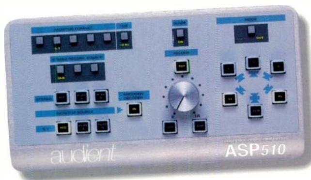
Audient's ASP510 surround controller provides one-knob level control for an active array of surround monitors (as well as one-touch speaker muting functions), and is therefore the box of choice at top-flight facilities such as London's Abbey Road. However, at a recommended UK price of just under £2000 including VAT, the ASP510 is harder to justify in the project-studio surround context!
