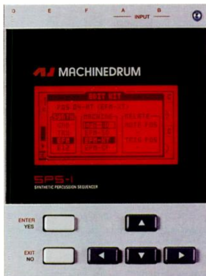
The SPS1's red LCD is packed with information, but this can make it a bit hard on the eyes if used for too long. Navigation around the multitude of options is via the cursors and Yes/No buttons.
