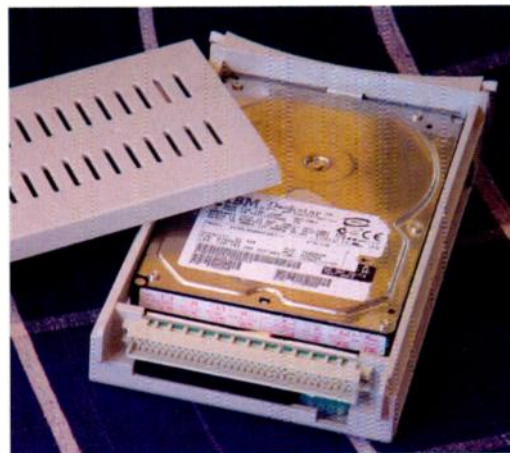
Once an IDE hard drive is mounted within a caddy, it can be inserted and removed from the Firedock in a matter of seconds, allowing true hot-swapping of hard drives.
