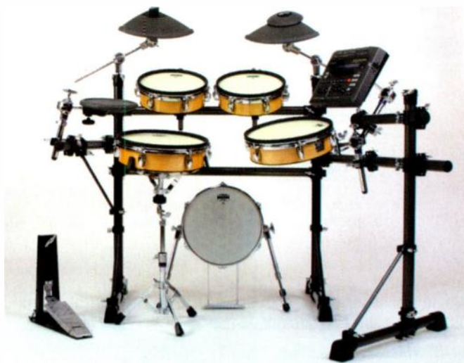
A set of drum trigger pads, such as this one from Yamaha, can be used to trigger artificial sampled sounds, while keeping something of a human feel in the rhythms.
