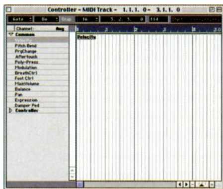
The Controller Editor. The left-hand pane shows the Controller types available for the selected Part (in this case a MIDI part), while the right displays any Controller data.
