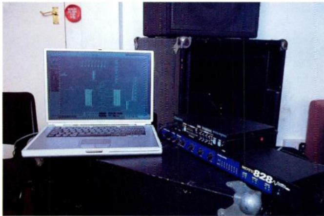
The new system: an Apple G4 Powerbook portable computer running Logic Audio and Unity DS1 , communicating with the outside world via a MOTU 828 audio interface and Micro Express USB MIDI interface.
