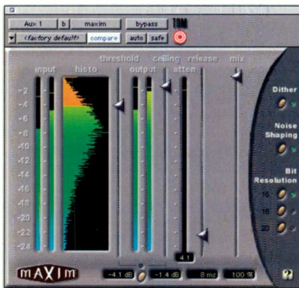
Figure 4: Digidesign's Maxim plug-in, a mastering processor that includes both maximisation and dither.
