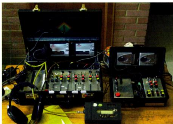
The two homemade mixers used for the recording sessions. The main mixer is on the left, with Frank Fox's The Box visual display above it, and the mixer on the right dealt with the feed from the Pearl DS60 microphone, allowing it to be used in place of an M&S stereo pair. Also in shot are the portable master DAT recorder, backup Minidisc recorders, and Sennheiser HD600 monitoring headphones.
