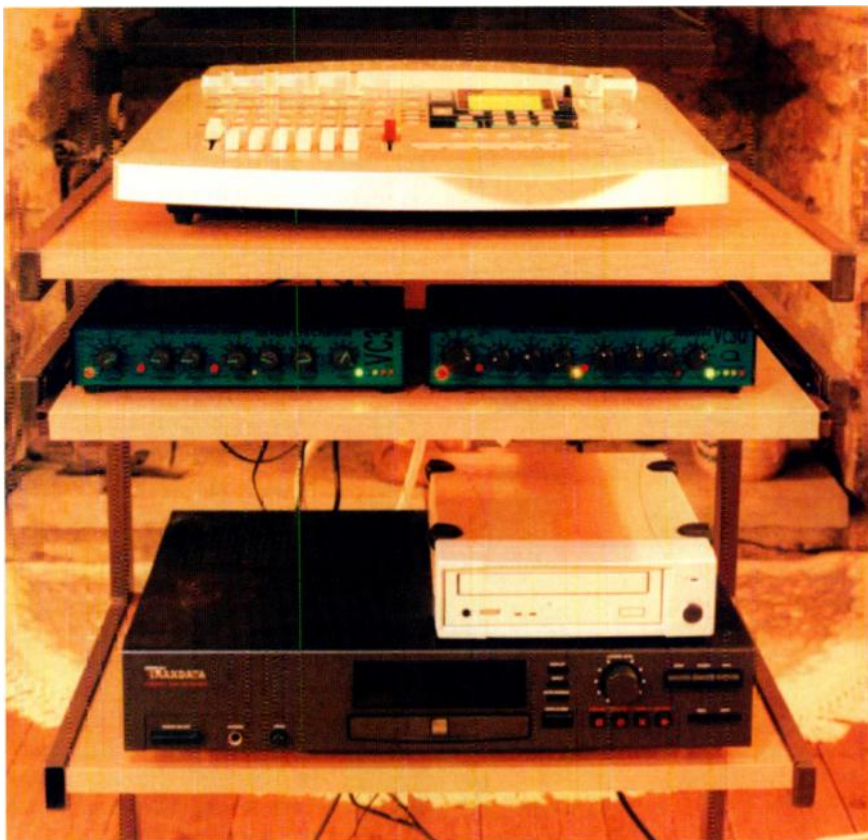
Almost everything Gary needs fits on a small mobile trolley: his Tascam digital eight-track, Joemeek VC3 preamps, and CD recorders. Gary has even recorded in stereo direct to the Traxdata CD recorder on location.
