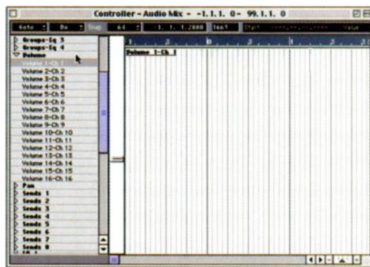
Cubase's automation data is stored in a single Audiomix Part for the entire Song, so data for all the VST Mixer Channels is available in the same Controller Editor window.
