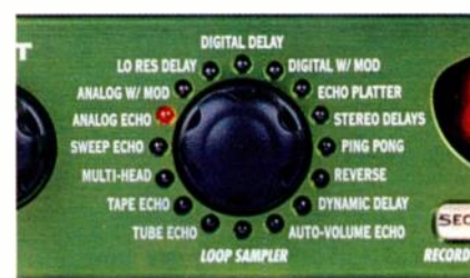
The Echo Pro models a variety of vintage analogue and digital delay processors, as well as offering a few original Line 6 treatments and a Loop Sampler.
