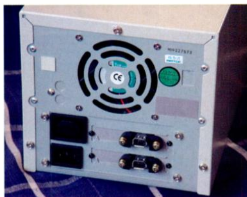
The external Firedock models provide two Firewire ports, allowing you to chain devices on a single Firewire buss.
