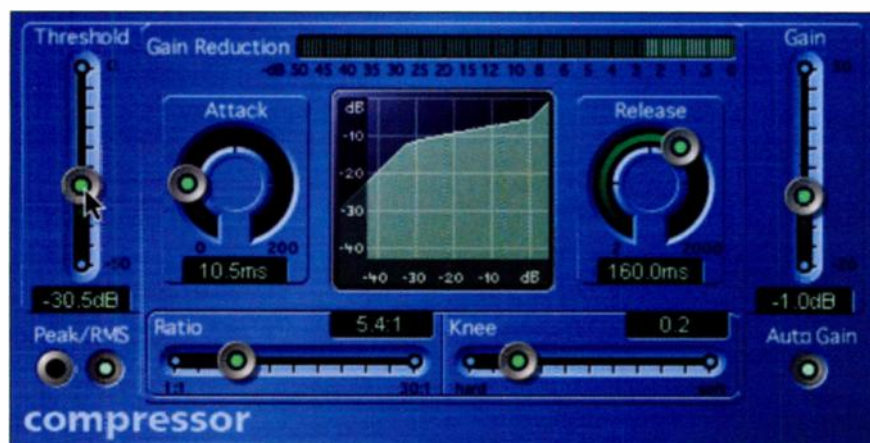
A useful general vocal compression setting is shown above, although again you'll need to adjust the Threshold to taste.
