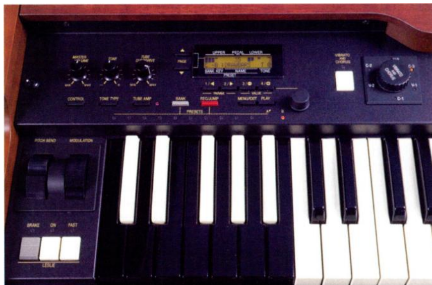
The complexities of the VASE tonewheel modelling engine have to be dealt with via the two-line LCD and menu-driven operating system, but otherwise the controls are either fairly self-explanatory, or like those of a real Hammond. The pitch-bend and mod wheels might seem out of place on a Hammond, but they're useful when controlling other sound sources via MIDI, or can also be assigned to virtual tonewheel speed and Leslie speed if you wish.
