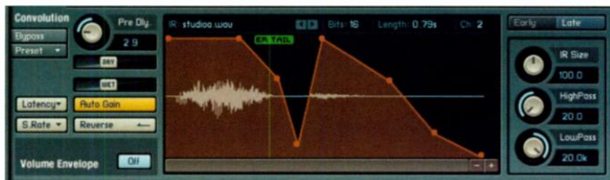
A convolution reverb, showing the optional eight-stage amplifier envelope.
