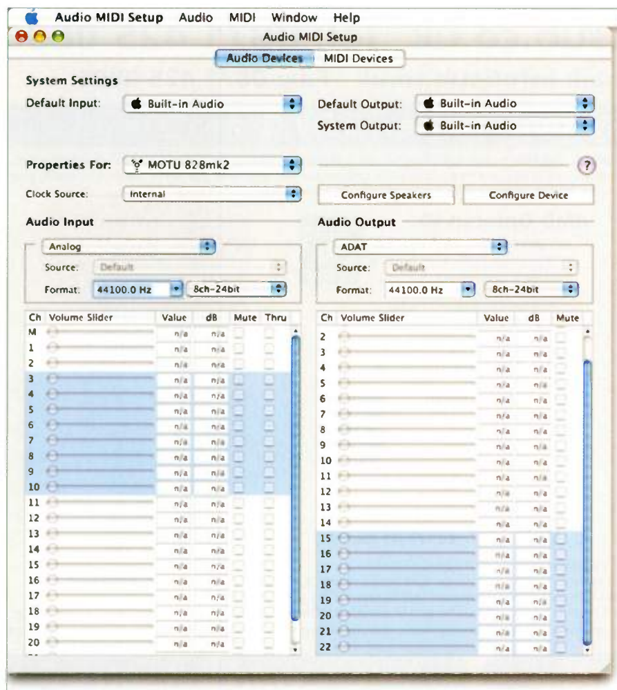
The Audio Input and Output properties for the Audio Device selected in the 'Properties For' pop-up menu are listed in the lower part of the Audio MIDI Setup application's Audio Devices page. Notice how the background for the channels contained in currently selected input and output Streams are highlighted with a blue background: using a MOTU 828 MkII, the Analog stream is selected for the Input and the ADAT stream is selected for the Output.
