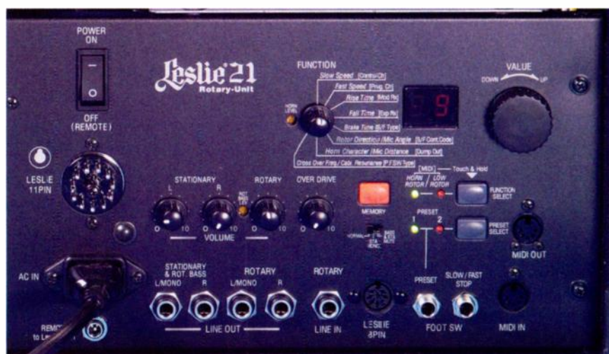
The involved connection panel of the Leslie 2101. There are four inputs, one of which comes via the quarter-inch input jack, while the others are carried via the 11-pin connector. The digital Leslie simulator is controlled by the buttons, knob and Value dial on the right. Footswitch and MIDI control is also available, and the knobs in the middle govern the output levels of the stationary speakers, the rotary horn, and the rotary amp's overdrive. The four outputs are at the bottom.
