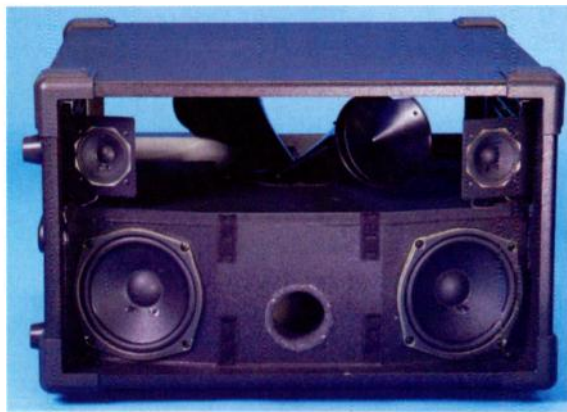
The 2101 with its grille removed, revealing the treble horn, five-inch woofers and two-inch tweeters.
