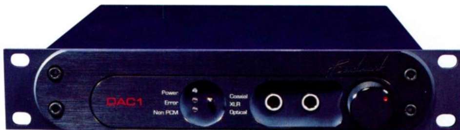
The DAC1's front panel has few features, although more than many D-A converters! The main one, on the right, is the large output level control. The recess in the centre contains a switch that determines the connector used on the rear panel for incoming digital audio, whether co-axial, XLR or optical. To the left of this are three status LEDs. The main two jacks are headphone outs driven by the dedicated internal Benchmark headphone amplifier.
