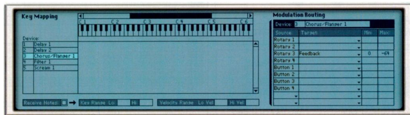
Screen H: Assigning the CF101's Feedback control (governing flange amount) to Rotary 3 on the Combinator .
