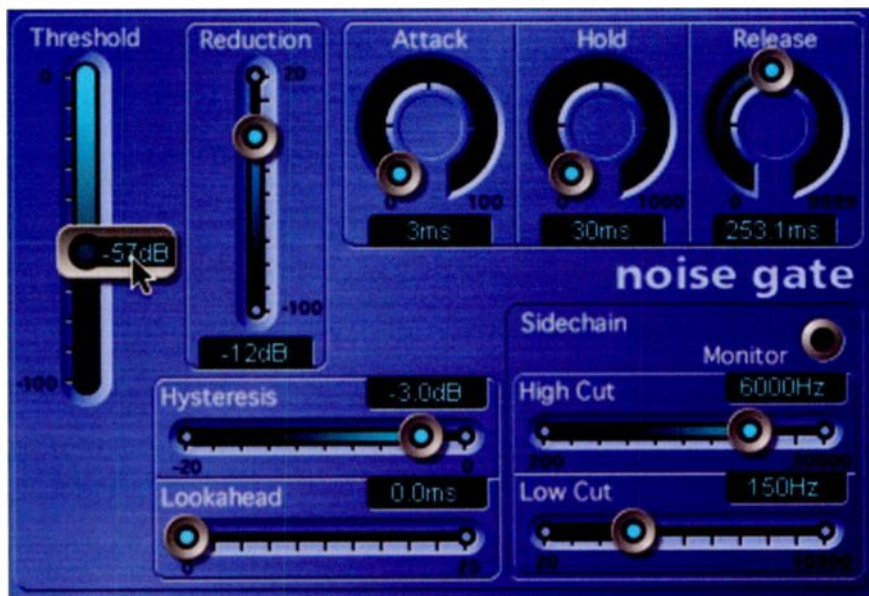
Here is how the Noise Gate plug-in might typically be set up for vocal processing. Threshold control would have to be set up by ear for each individual track so that the gate only operated during gaps in the singing.
