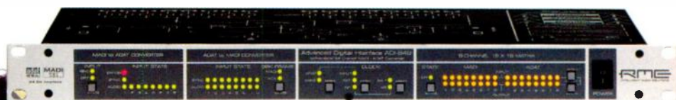
RME's Hammerfall DSP MADI card (left), combined with the ADI648 MADI-to-ADAT converter (above), makes for a powerful I/O system capable of handling up to 64 simultaneous channels.
