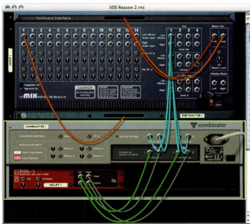
Screen C: Re-cabling the Combinator 's main ins and outs for send-and-return operation.
