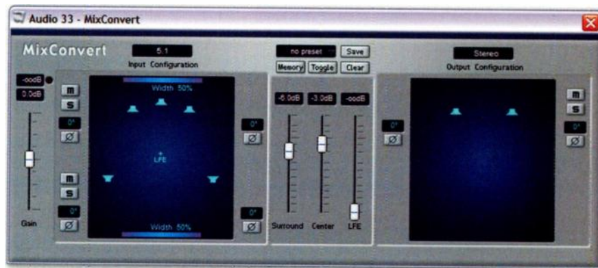
Nuendo 3 includes a new plug-in called Mix Convert to make it easy to downmix files, as shown here, to create a stereo mix from a 5.1 source.
