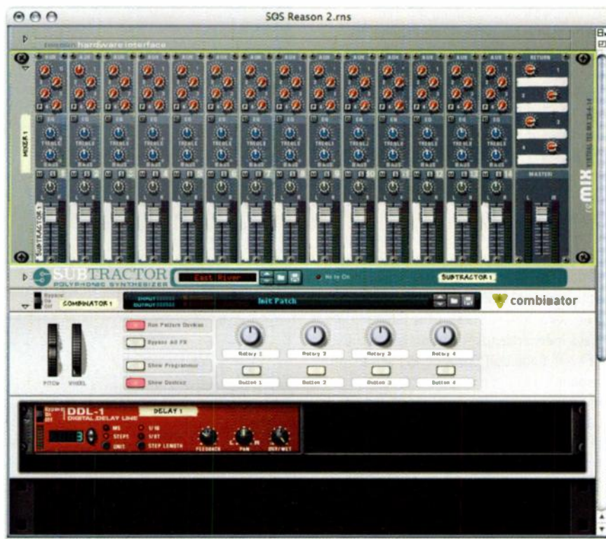
Screen B: The basic starting rack, featuring mixer, synth and Combinator . A DDL1 has been placed inside the Combinator .
