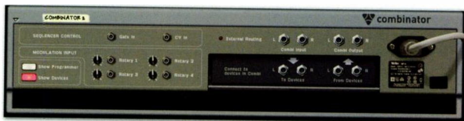
Screen A: The Combinator 's rear-panel connections. Note the separate sockets for passing signal to and from the devices inside the Combinator .
