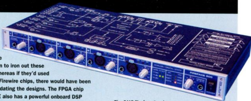
The RME Fireface 800 has an updatable Field Programmable Gate Array (or FGPA) chip at its heart, like the recent MADI-enabled Hammerfall card.
