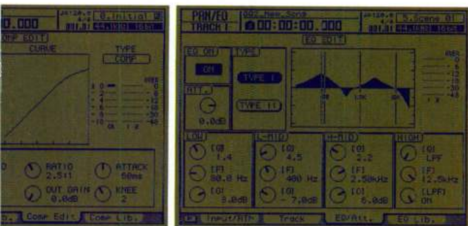
The main Channel View screen (far left) allows you to see at a glance how all the processing is routed for each channel. Separate screens (left to right) then provide detailed settings for the gate, compressor, and EQ.
