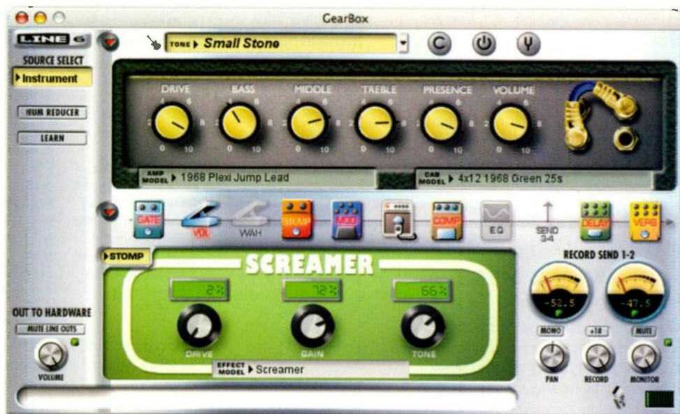
The Gearbox software in action. The row of icons along the middle shows the signal path from left to right, with the selected amp model displayed above, and the effects displayed below.
