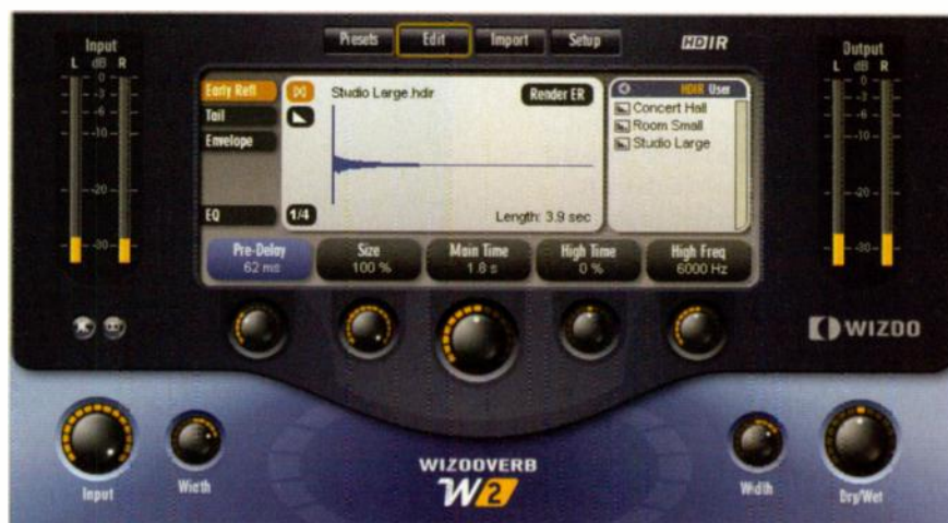
One of W2's unique features is the ability to 'render' IR-based early reflections and tails to a synthesized equivalent for greater flexibility.
