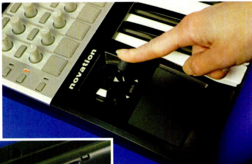
The 25SL has the innovative joystick controller seen on previous Novation Remotes; its action can be sprung or not, depending on how you set the sliding switch on the underside of the unit (see left).
