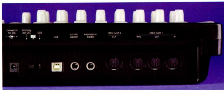
The 25SL can be powered by batteries or over USB. Other than that, the connectors are fairly standard, with two MIDI ports, the USB socket for connection to your computer, and sustain- and expression-pedal jacks.
