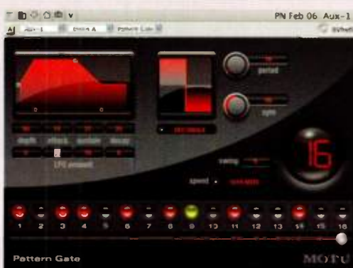
Because of its automatable envelope generator and on-board LFO, the Pattern Gate plug-in can do a lot more than 'stuttering' effects.
