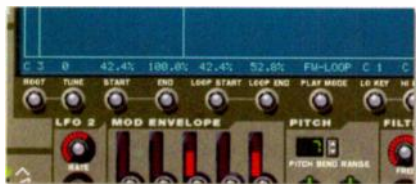
The Start, Loop Start, Loop End and Play Mode controls are the keys to providing looped playback.
