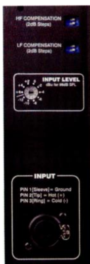
Above its rear-panel combi-jack/XLR input, the S7 carries HF and LF frequency-tailoring switches and an input gain trimmer.
