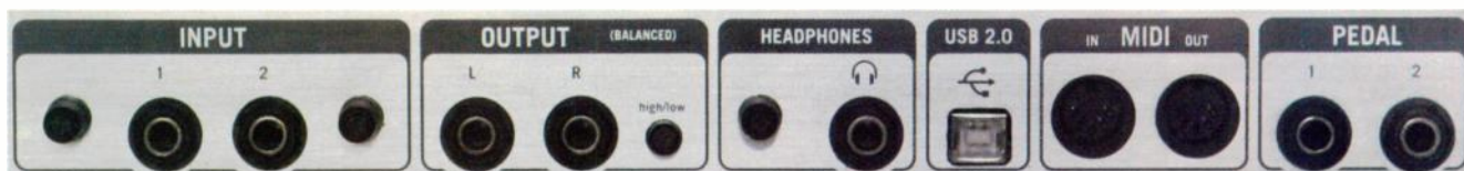
The new Rig Kontrol 2 is a USB 2 audio and MIDI interface as well as a guitar-optimised DI box.
