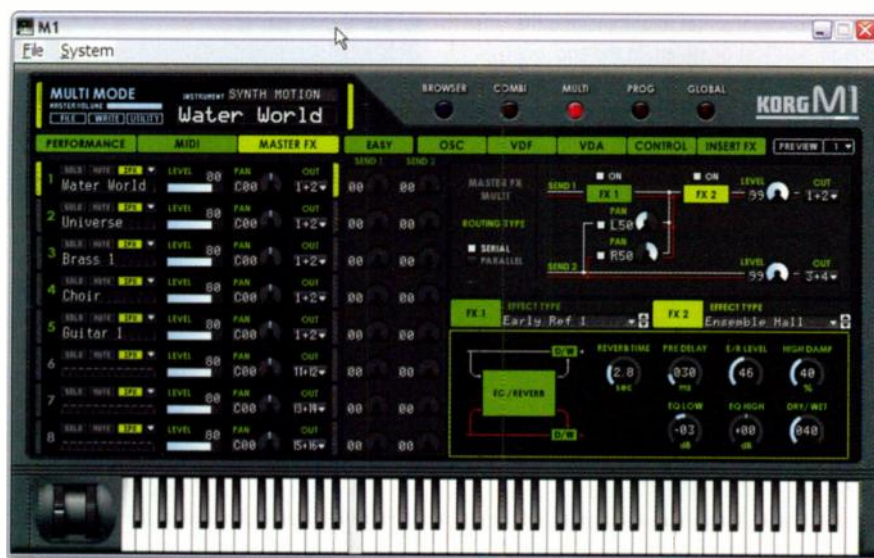
The new Multi mode is a supercharged multitimbral Combi with up to eight Programs (each with two Insert effects), assignable to a maximum of eight MIDI channels and eight stereo outputs.
