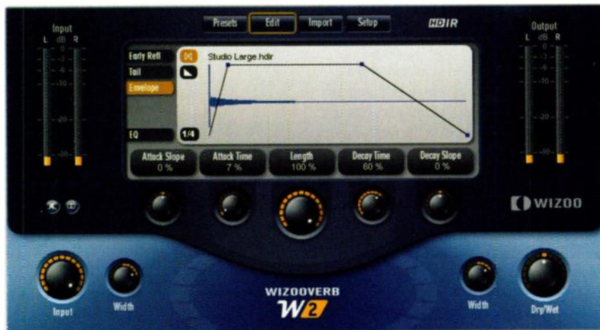
Reverb tails generated from an impulse response can be modified using the Envelope tab.
