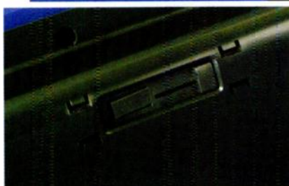
The 25SL has the innovative joystick controller seen on previous Novation Remotes; its action can be sprung or not, depending on how you set the sliding switch on the underside of the unit (see left).
