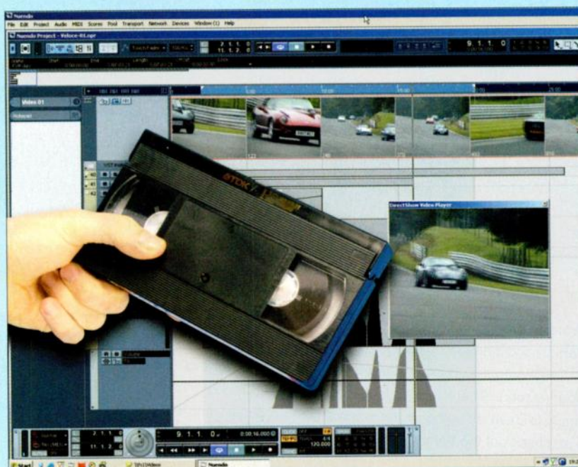
Until a couple of years ago, most music-for-picture jobs were supplied on humble VHS cassette, which necessitated slaving a VCR to a sequencer with a synchroniser — in the author's case, a MOTU MIDI Time Piece AV. Recently, though, most video has been supplied as AVI or Quicktime files on CD-ROM and can be run directly within a software DAW such as Nuendo (shown above).
