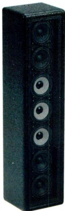
■ The EAW CLA37 column loudspeaker uses seven 3-inch drive units to achieve a coverage of 120 degrees horizontal x 30 degrees vertical, thus controlling the vertical dispersion tightly. It is suitable for speech reinforcement in large reverberant environments if several or many units are distributed amongst the listeners.
