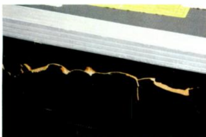
❏ This flightcase was designed to hold audio-visual display equipment, not PA gear. The damage has been caused by a heavy object moving around inside.
