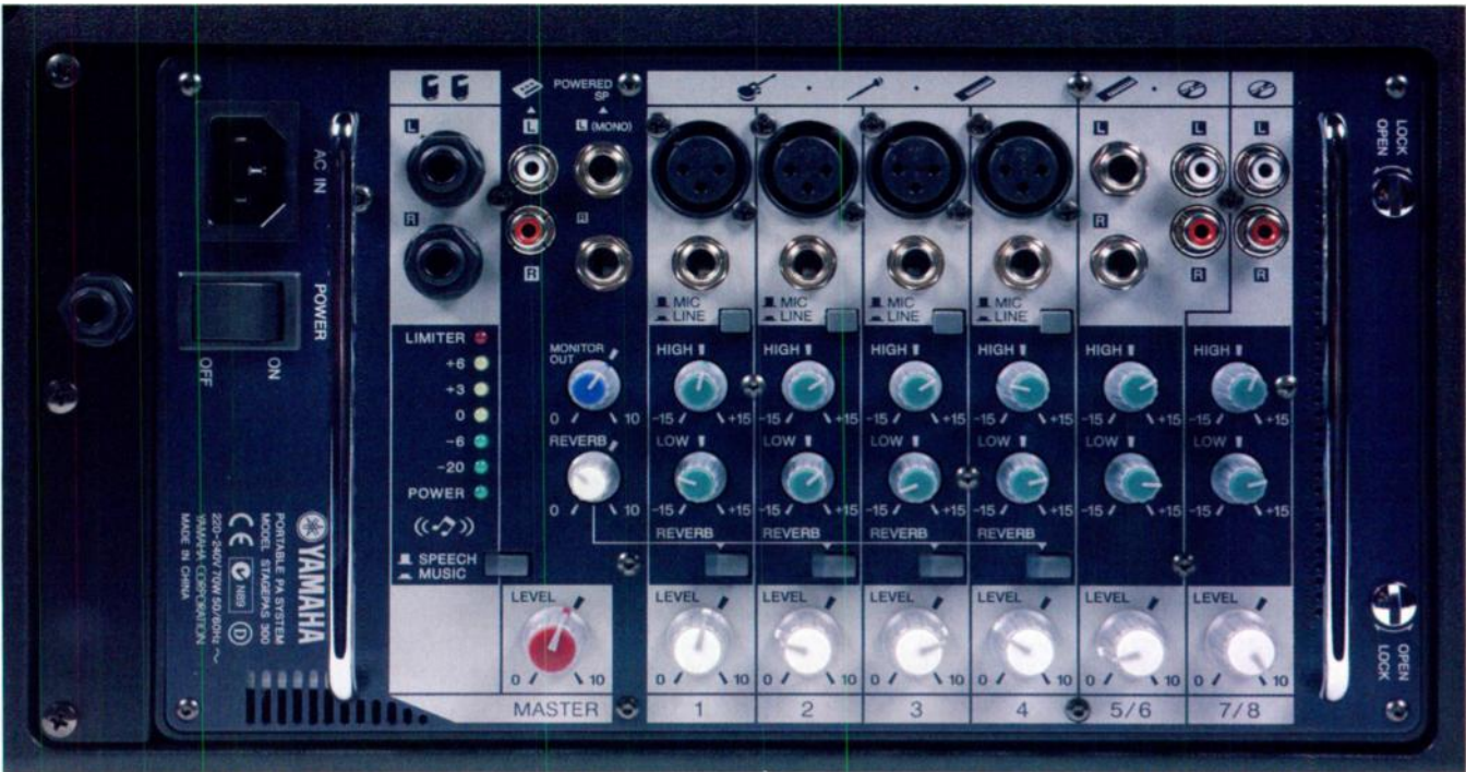
3 The mixer offers four mono mic/line channels which can each access the basic built-in reverb (but not in variable amounts), plus two stereo channels offering jack and/or phono inputs. High/low EQ is available to all channels. Other features include jack outputs for connecting powered monitoring and a pair of phono recording outputs.
