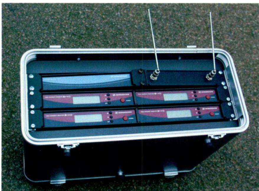
❏ A metal 19-inch rack case safely housing a set of radio-mic receivers.
