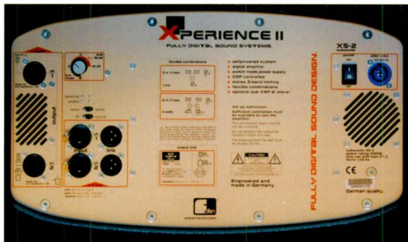
▲ The subwoofer is the business end of the Xperience II system, containing a pair of 500W amplifiers and the DSP for EQ and limiting. The rear panel of the sub features all inputs and outputs, Powercon mains power inlet and power switch, ground-lift switch, and LEDs to show signal presence/clipping and whether speaker protection has kicked in.
