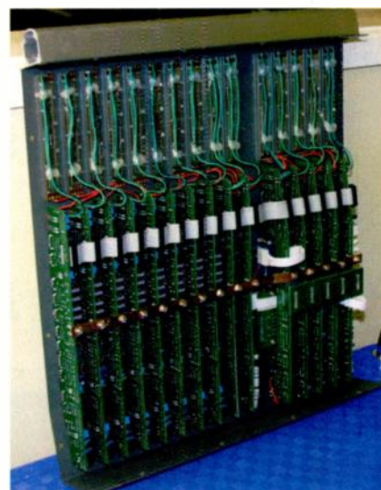
■ A view of the individual circuit boards used for each channel.
