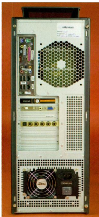
As well as the rearward-pointing grilles, this PC is also ventilated via the top of the case.
