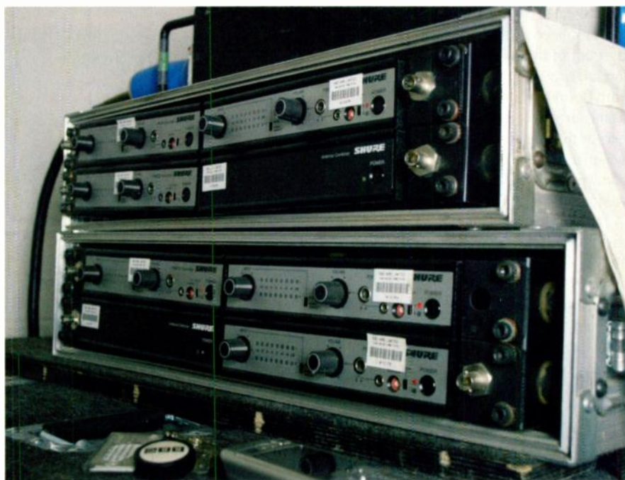
■ A mixture of in-ears and wedges are used on TOTP for monitoring. This rack contains Shure PSM700 in-ear receivers.
