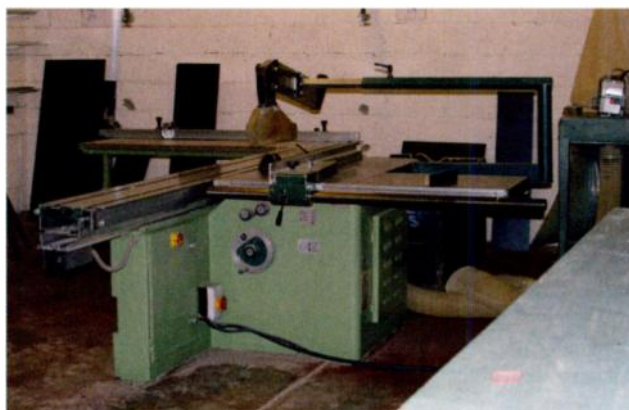
❏ A cutting machine used on the boards that form the panels of the flightcases.
