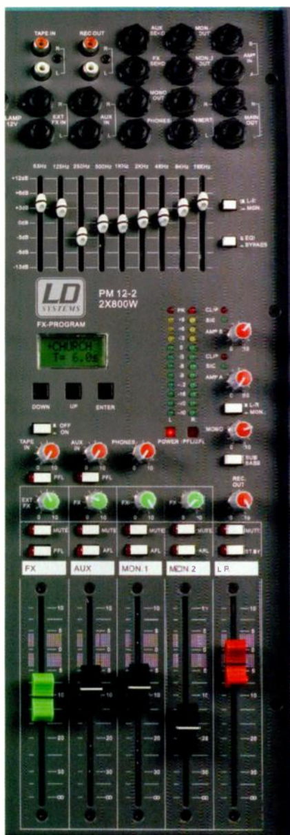
▲ The Master (bottom), effects (centre) and graphic EQ sections of the PM 12-2.
