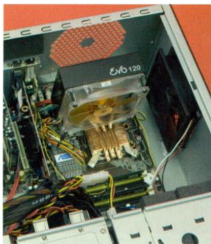
The Akasa Evo 120 CPU cooling system, with its large fan, is becoming a popular choice in PCs where low noise is important.
