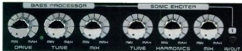
The SX3040 Sonic Exciter has two identical, independently operated channels. Each is divided into two sections: the first filters off and processes the bass (using compression and automatic phase-shifting); while the second is used to enhance the higher frequencies by adding extra harmonics.
