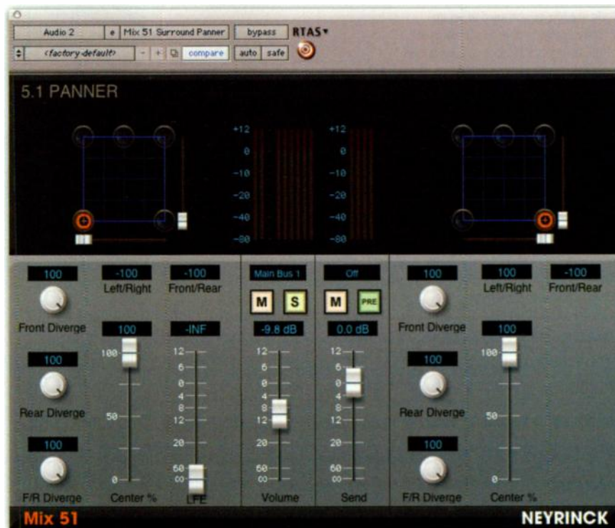
The stereo Surround Panner is, in most respects, a dual-mono design, and doesn't allow you to pan both channels with a single movement.
