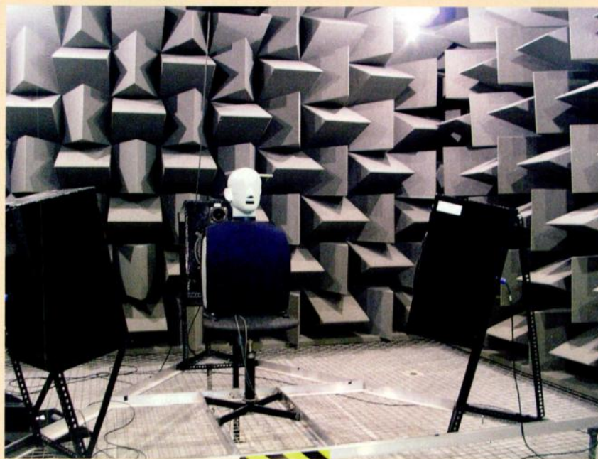
Creating HRTFs is a complex and expensive business. Here at Salford University, a dummy head is placed in an anechoic chamber and test tones are recorded from strategically placed speakers.
