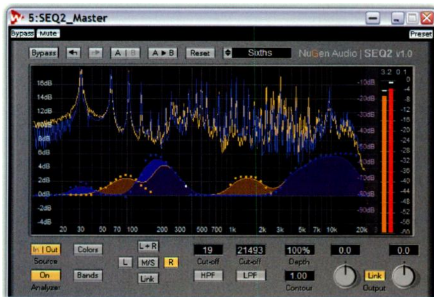
Drawing in a suitable EQ curve using SEQ2 is easy and painless, while the integral spectrum analyser helps you spot problem areas that need treating.
