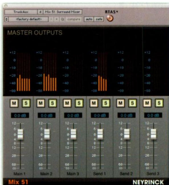
The Surround Mixer plug-in can address up to three main 5.1 and three quad send buses.
