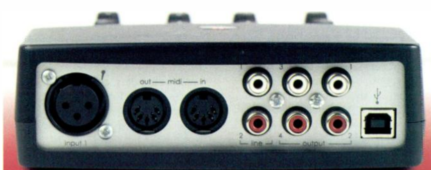
The Nio's rear panel, sporting most of the unit's I/O. Input 2 and the two headphone sockets can be found on the front and three switches on the right-hand side set input impedance level and turn Input 1's phantom power on or off.
