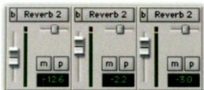
If you have the sends in Pro Tools' Mix window set up to display the level and pan sliders, pressing a Command 8 Send button in Console View will switch to the appropriate send in the Mix window.
