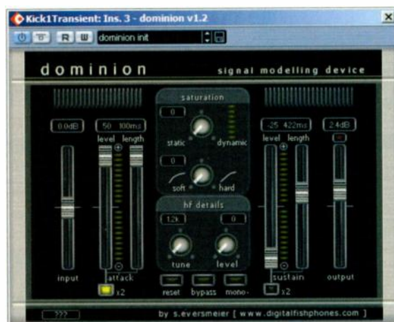
The low-end punch of one of the two kick-drum samples was improved with a low-pass-filtered Digital Fishphones Dominion send effect.
