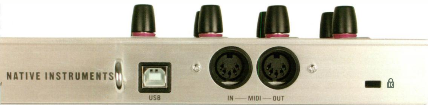
The rear panel of the Kore 2 controller — now without audio connections but with an extra pedal socket.
