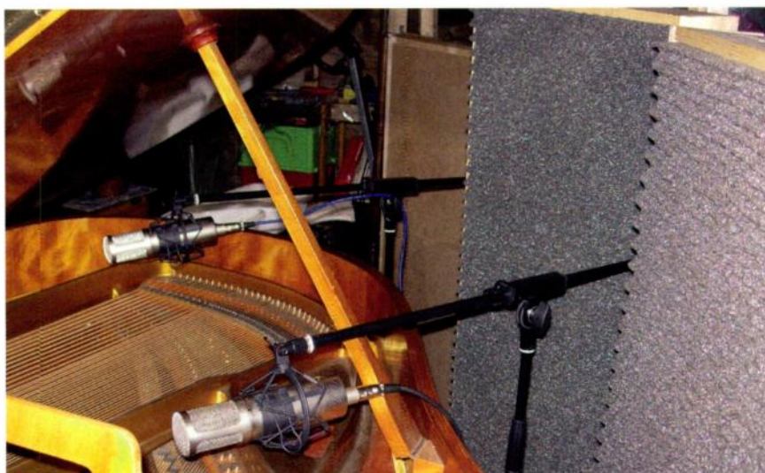
A spaced pair of Studio Projects C3 mics were used to capture the piano sound, while four acoustic absorber panels were arranged to try to reduce spill from the drums.
