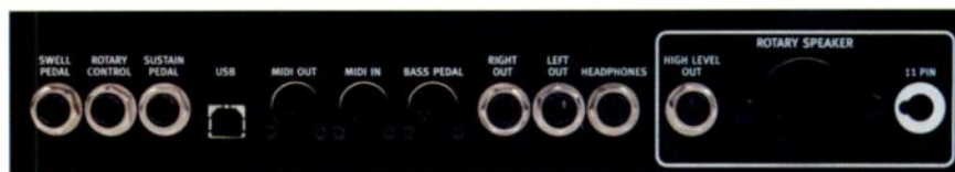
The C1's back panel: note the unusual selection of MIDI ports.
