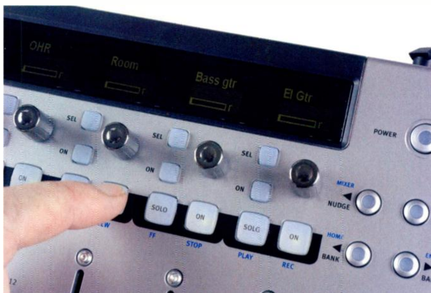
With no dedicated transport controls, the Solo and On buttons for the last four channels double in this role.
