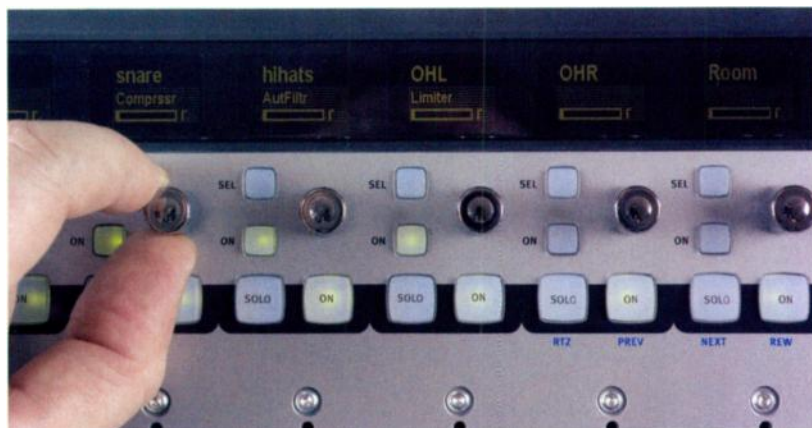
In Insert mode, each display shows the contents of a single plug-in slot on its associated channel; if Channel mode is active, the eight channels show the first eight plug-in slots on the 'attended' channel.
