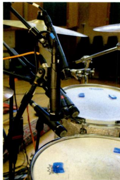
To give some idea of the kinds of tonal change that fine positioning can bring about when using a snare-drum close mic, we set up six different Shure SM57s as shown here, generating the 'SnareTopPos' audio files.
