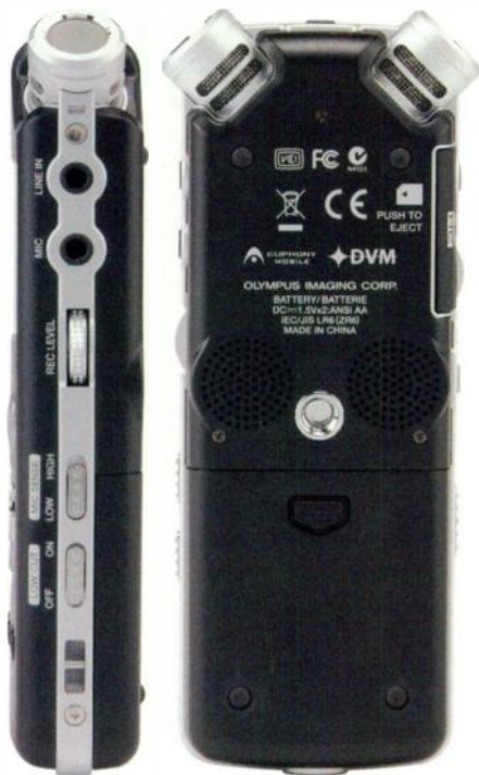
The battery compartment is found on the LS10's rear panel, where there's also a camera tripod thread and some small playback speakers. The mic and line inputs, a high-pass filter and mic-sensitivity and recording-level controls are found on the right-hand side.
