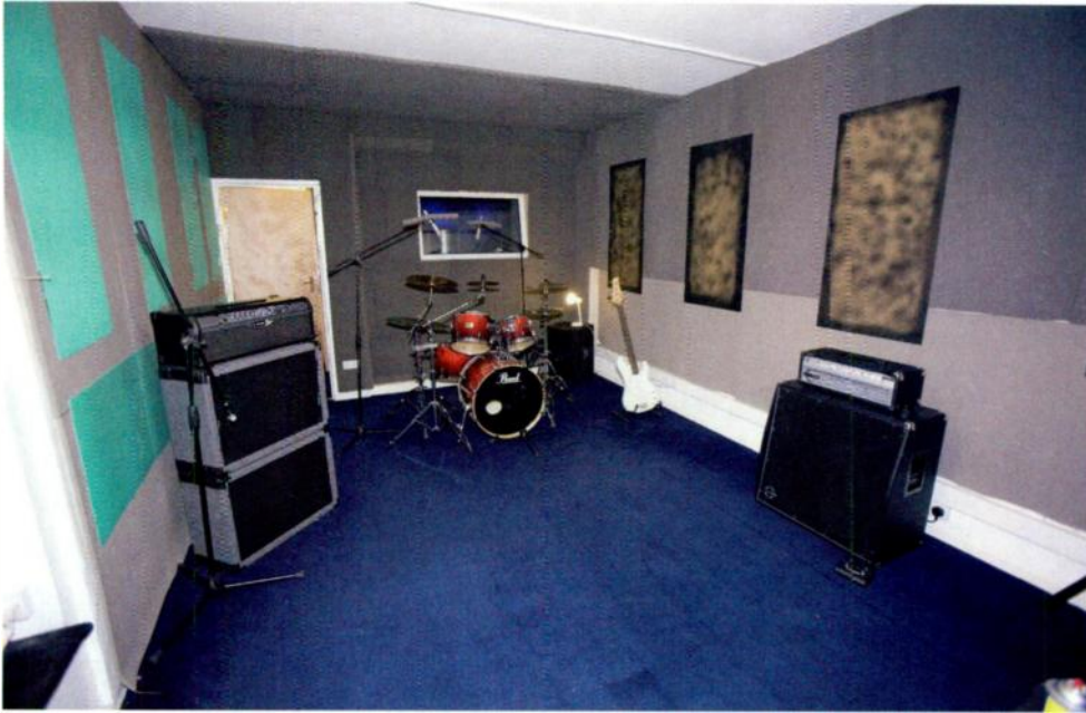
Using a combination of plastic sheets and MDF panels, some high-frequency reflections were added back to the live room, without compromising the absorption of mid and low frequencies.
