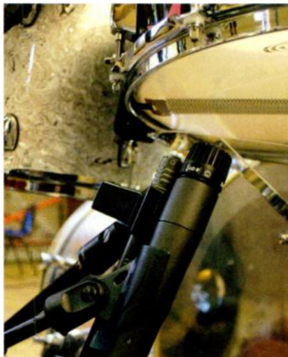
Five classic snare mics were compared over the top of the drum for the 'SnareMics' audio files (left, clockwise from top left): a Neumann KM84, a Shure SM57, an AKG C451EB, a Neumann KM86 and an AKG C414B-ULS. Above, under the snare were a further SM57 and C451EB.
