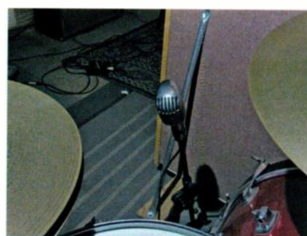
Gabe Roth's favoured single-mic placement for recording drums, with a Shure 55 between kick and snare; above, from the drummer's point of view.
