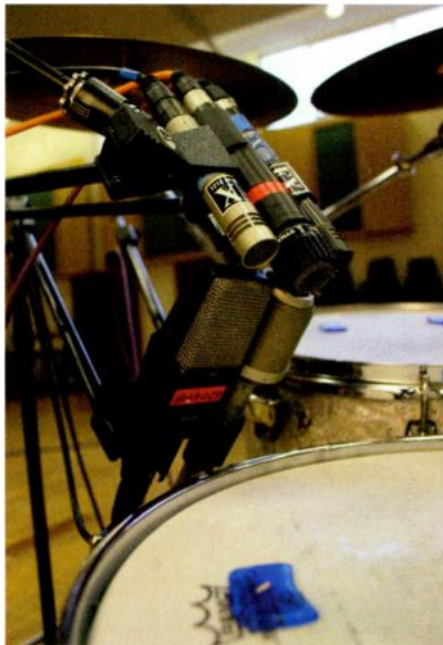
Five classic snare mics were compared over the top of the drum for the 'SnareMics' audio files (left, clockwise from top left): a Neumann KM84, a Shure SM57, an AKG C451EB, a Neumann KM86 and an AKG C414B-ULS. Above, under the snare were a further SM57 and C451EB.
