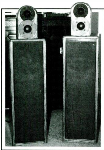
PHOTO 1: The cabinet on the right is resting on homemade spikes; the cabinet on the left is flat on the carpet. The spikes' appearance is subtle.
