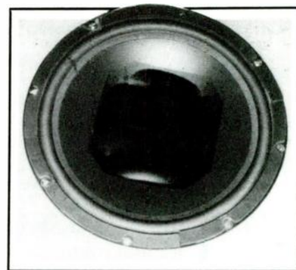
PHOTO 2: "Gooped" woofer with black contact paper cover.
