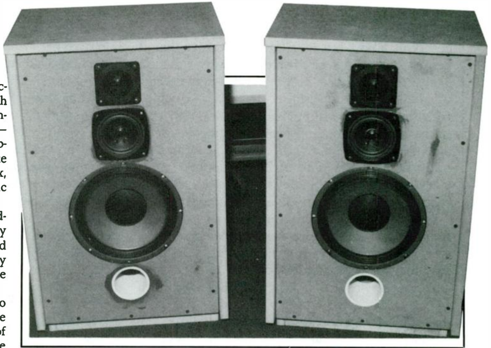
PHOTO 1: These loudspeakers were constructed of fiberboard according to the author's plans, but the front panel is recessed, the top panel is slightly wider, the port is below the woofer and the base is larger. The drivers are those recommended in the parts list.
