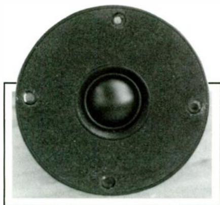
PHOTO 1: The original tweeter with foam rubber covering.
