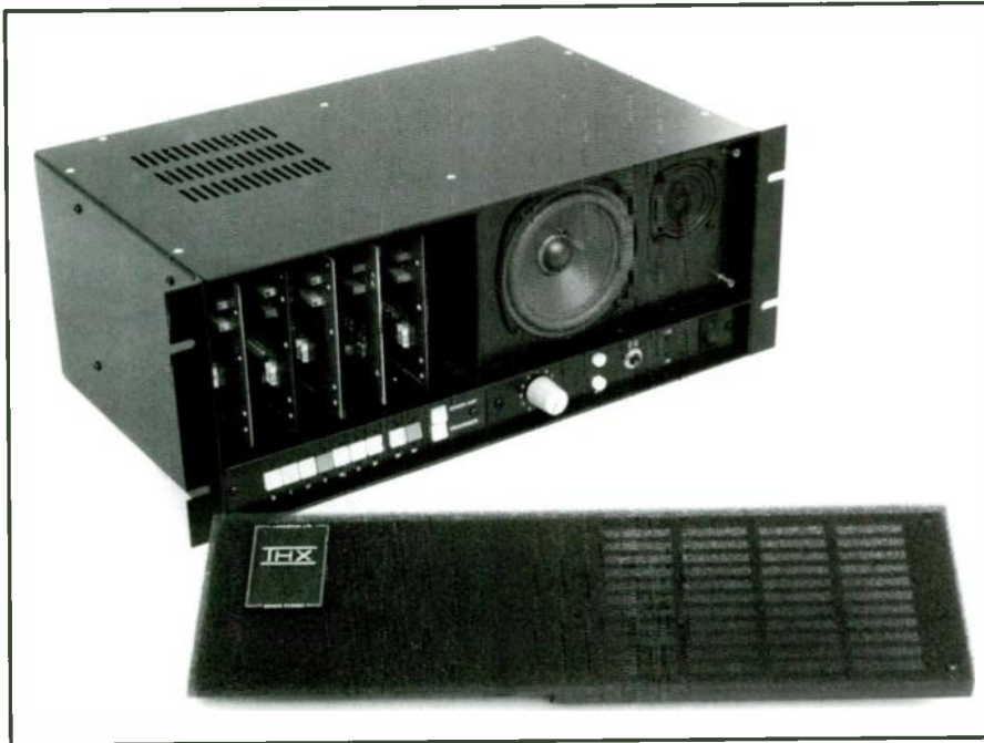
PHOTO 3: THX crossover boards and monitor control panel. Shown is a five-channel system in a rack that allows monitoring each channel's crossover and amplifier output.
