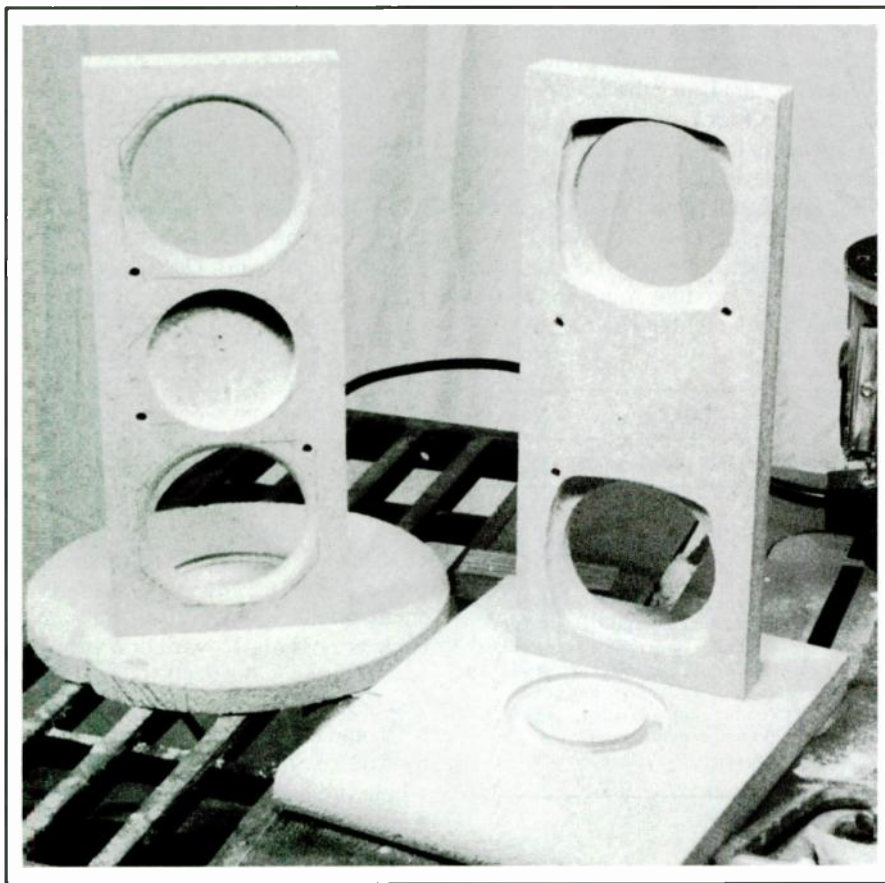
PHOTO 6: The internal baffle boards, completely machined and ready for installation. Note the position of the three 1/4-inch lead wire holes on each baffle.
