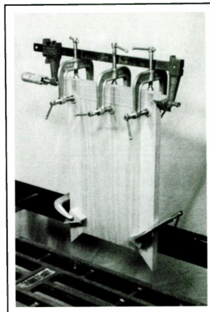
PHOTO 1: Miter that joint. Four clamps hold the facing firmly in position.
