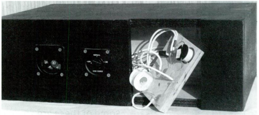
PHOTO 1: Crossover in the open back of the enclosure.
