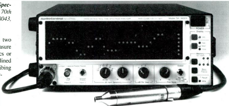
PHOTO 1: AudioControl's Model SA-3050A third-octave real-time spectrum analyzer.
