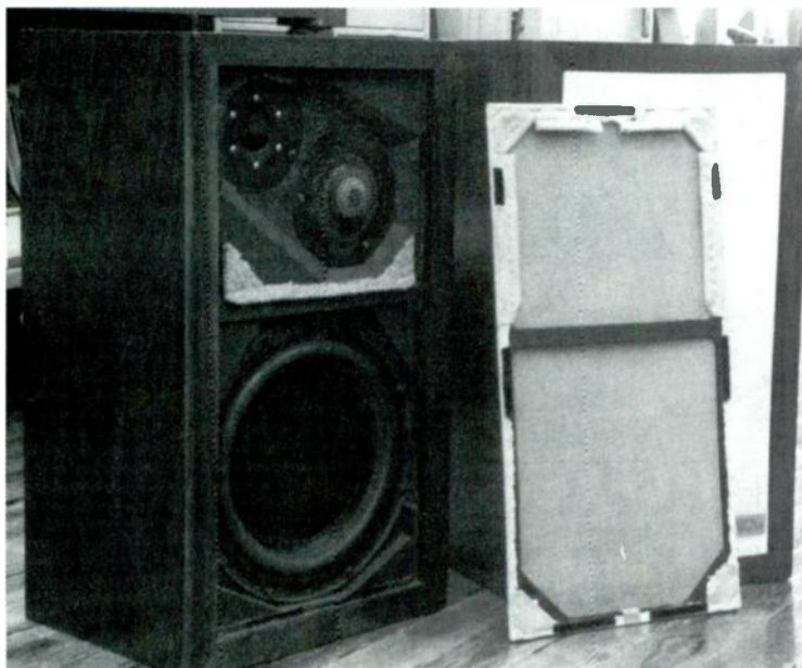
PHOTO 1: The finished product. Note the stock appearance until you remove the grille. The foam-filled woofer cone, baffle amendments, new treble facia, and felt stapled to grille frame are visible.
