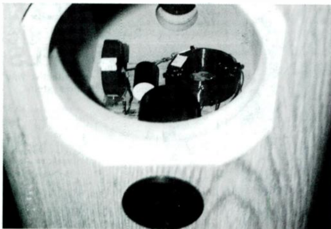
PHOTO 3: Woofer crossover installed.
