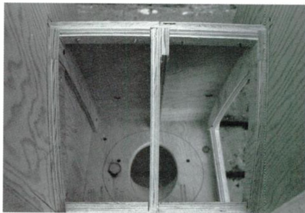
PHOTO 10: Rear horn plate installed.
