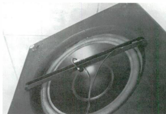
PHOTO 2: Closeup showing mike-mounting detail.
