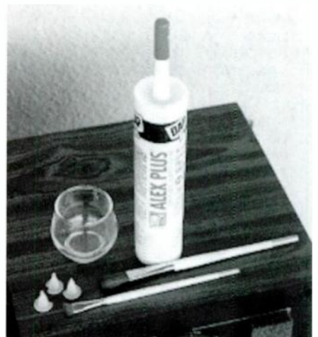
PHOTO 2: The materials used are few. The brushes are artists brushes by Duncan, but this quality is not required. The plastic plugs are inserted into the frame's mounting holes to elevate the frame and surround when the driver is facing down.
