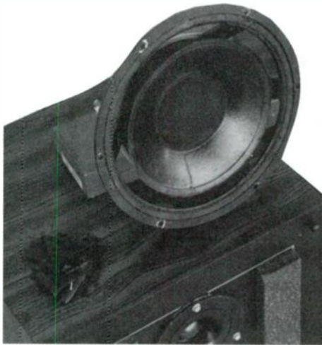
PHOTO 1: The original Dynaudio 21W54, a superb 8" driver, rendered useless from foam rot. Its surround had completely disintegrated as a result of long use and exposure to high heat levels. Every piece of the surround had broken free at the cone and frame junctions and collected at the bottom of the grille frame.
