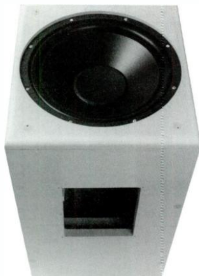
PHOTO 11: Enclosure with trim plate and woofer.
