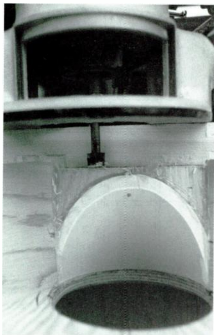
PHOTO 8: Trimming the reflector-cap height.
