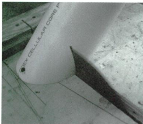
PHOTO 7: Cutting the throat reflector.
