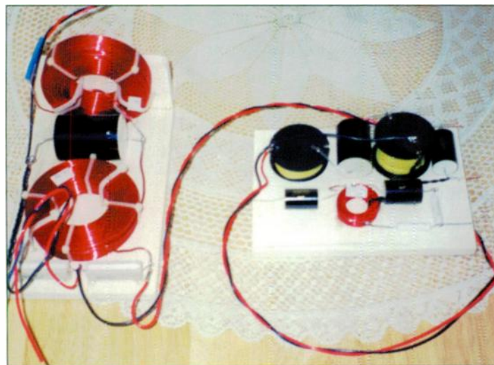
PHOTO 1: Low-pass crossover network (left), mid and high crossover network (right).
