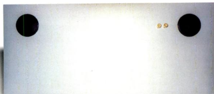
PHOTO 6: Rear view of cabinet. Note vent ports and Axon terminal posts.
