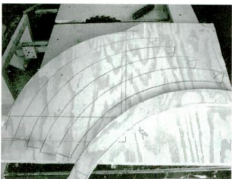
PHOTO 21: Tracing the large horn braces.
