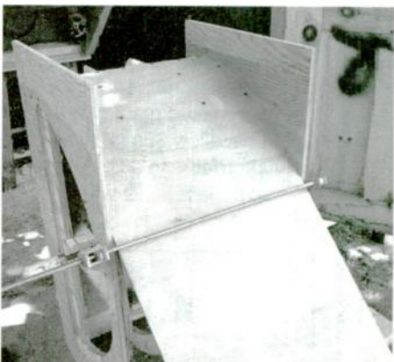
PHOTO 25: Holding the large horn panel in place during assembly.
