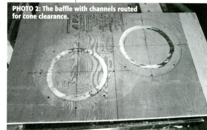
FIGURE 2: Baffle view; for clarity, not all parts or details are shown.
