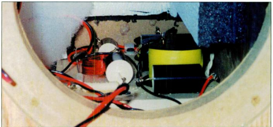
PHOTO 3: Mid- and high-pass crossover network mounted on right side.
