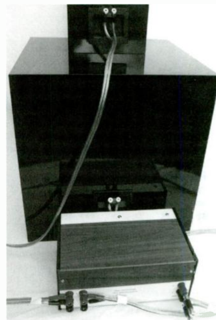
PHOTO 2: Crossover connected to speakers.
