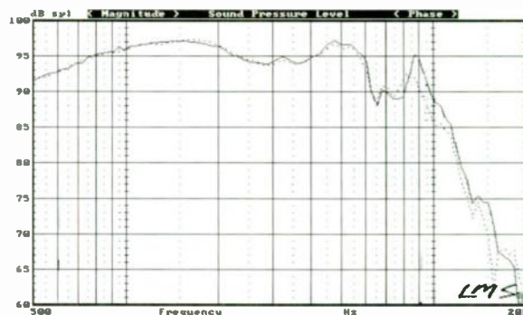
FIGURE 7: CSX 145 H SPL comparison for two samples.
