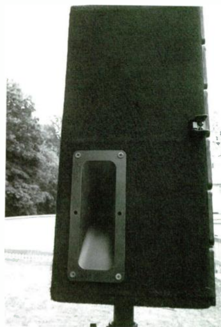
PHOTO 35: Side-fire tweeter aligned vertically to minimize interaction with the main array.
