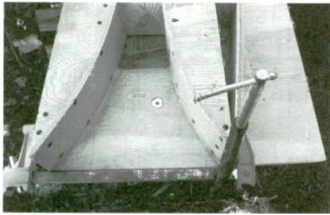
PHOTO 11: Using two clamps to bend a port horn plate into place while it is screwed to the small-horn assembly.
