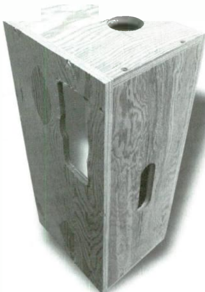
PHOTO 33: Holes in the high-frequency box for side-fire tweeter, pole-mounting socket, and handle.
