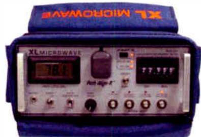
Each *Path Align-R™* (set of two) contains 4 bands (to 23.5 GHz) and is both a synthesized source, that *directly drives* the site's antennas, and a narrow-band receiver. The instruments provide continuous 2-way voice communication between antennas!
