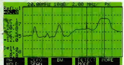
Fast, full function 5-860 MHz Spectrum Mode for tracking down ingress.
