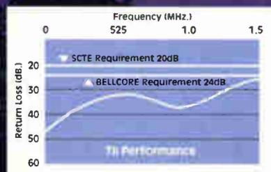
TII can handle high energy surges with very low capacitance and low arc voltage. Our coaxial protectors easily exceed both SCTE and Bellcore requirements. For more information, call 1-888-844-4720. Visit us at [www.tii-industries.com](http://www.tii-industries.com).
