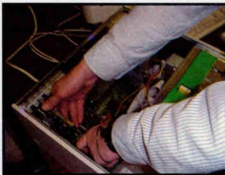
The installer inserts the NIC into an open expansion slot in the customer's computer. Note the grounding cord on the installer's left wrist, used to prevent damage to the equipment from static shock.
