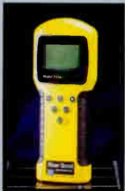
Riser-Bond Instruments' hand-held time domain reflectometer (TDR) locates faults in short- or long-range applications on all types
