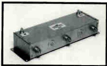
Microwave Filter's Model 13430 Bandpass Filter is designed to enhance test measurements by eliminating out-of-band (OOB) signals from the input of a spectrum analyzer, allowing cleaner measurement of the data portion of a transmit signal. The unit has a passband from 640-660 MHz and an insertion loss that typically is less than 1 dB. The group delay over the passband is less than 20 ns. A minimum of 40 dB rejection is achieved from 0.3-550 MHz and from 750-1000 MHz.
