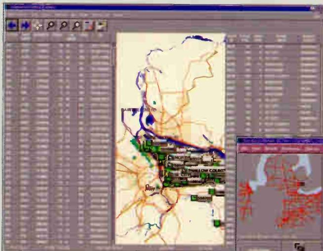
What the dispatcher sees: Above, Brazen's automated routing screen shows the dispatcher where all the day's jobs are, as well as their status. At right, the dispatch screen tracks the individual job status by time, location, work order, technician and several other variables. Screen captures courtesy of BrazenSoftware
