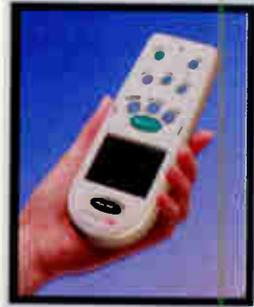
Interlink Electronics' Interactive Remote enables remote control of electronic devices, keyboard-less text entry and wireless telephony.
