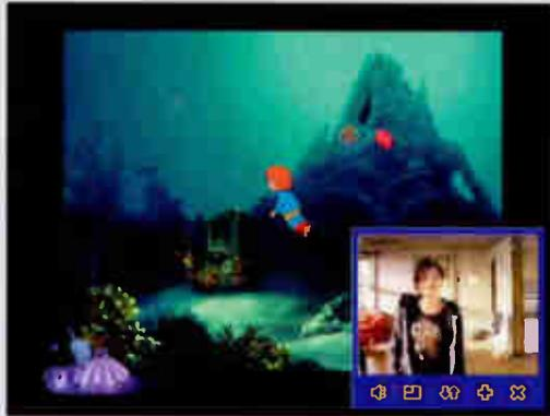
Subscribers activate the picture-in-picture feature via their single-tuner digital set-top box. Peach used Scientific-Atlanta's set-tops for the demo. The video channel they select is fed to new Interactive Media Server software. The IMS digitizes the video, compresses it to a lower bit rate, combines it with computer output into a single
