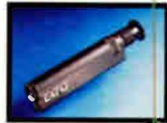
Delivering 400X magnification, the Fiber-Optic Microscope also detects flaws from factory non-specification errors, shipping and handling problems, and other situations prior to connectorization. EXFO offers the 'scope for use as a self-contained handheld as well as a component in several test kits for outside plant use. The instrument comes in a casing intended for field use.
