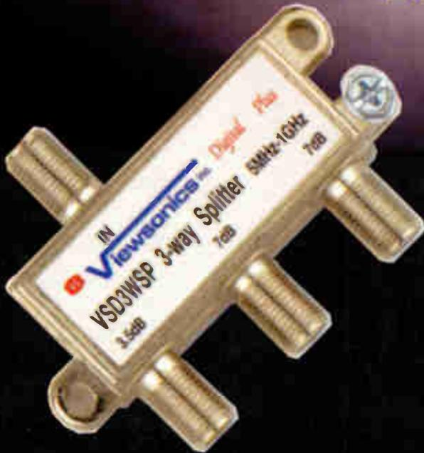
Viewsonics has created the Digital Plus line of passives to meet the increased demands of CATV operators for inter-modulation protection. Along with capacitive protection from transient voltages, the Digital Plus line incorporates improved ferrite design that maintains linear properties in high signal level environments even after suffering a high voltage surge.
