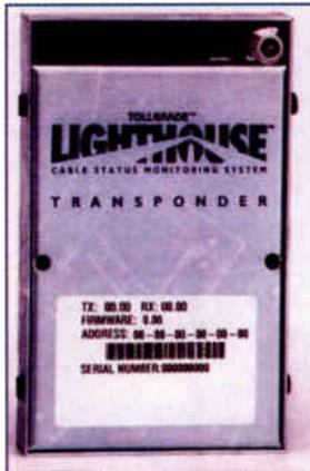
The Tollgrade 135PSM1 transponder is designed to provide power supply monitoring and control over a hybrid fiber/coax (HFC) network. Part of Tollgrade's Lighthouse Cable Status Monitoring System product suite, the unit is dynamically frequency agile in both directions, from 5-15 MHz for the return path transmitter, and from 50-135 MHz for the forward path receiver. The transponder monitors individual battery voltages
