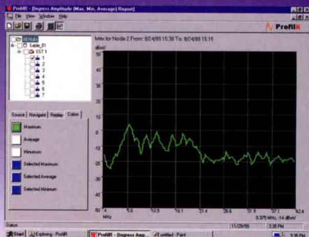
*TrafficControl™ measures and plots ingress spectra of bands fully occupied by return traffic*
