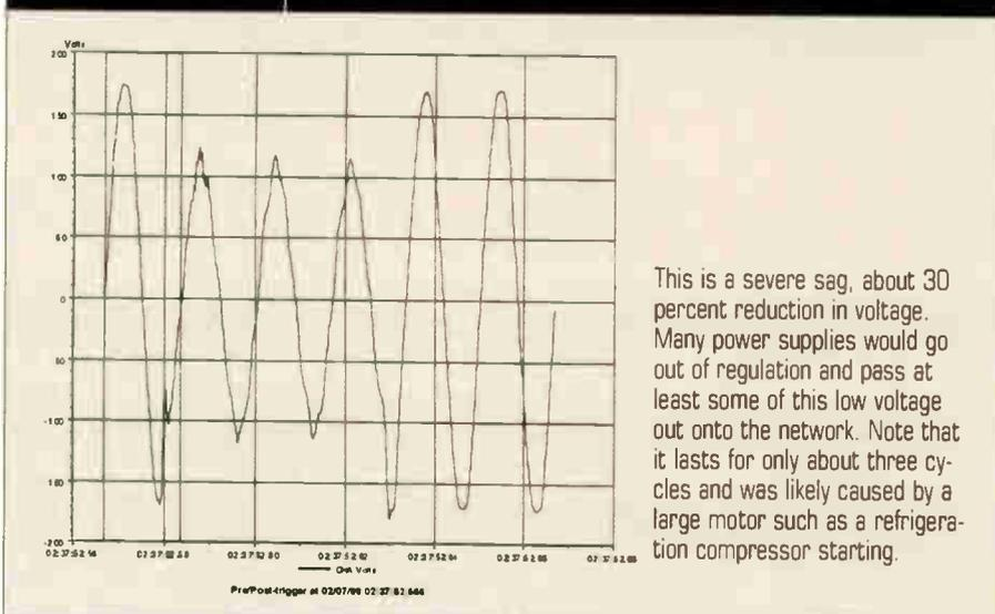
This is a severe sag, about 30 percent reduction in voltage. Many power supplies would go out of regulation and pass at least some of this low voltage out onto the network. Note that it lasts for only about three cycles and was likely caused by a large motor such as a refrigerator compressor starting.
