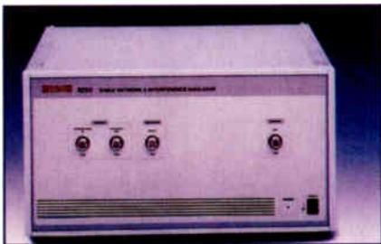
The Telecom Analysis Systems 8250 emulates hybrid fiber/coax (HFC) cable network impairments in a controllable laboratory instrument. This cable network and interference emulator is designed to evaluate the transmission performance of cable modems, cable modem termination systems (CMTSs),
