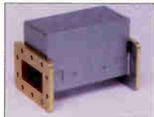
Microwave Filter Company's model 7892D waveguide band-pass filter suppresses strong out-of-band (OOB) interference caused by marine or airport radar systems. The filter has a typical insertion loss of 0.5 dB at the center frequency and 1.25 dB maximum (1.0 dB typical) at 3.7 GHz and 4.2 GHz. Suppression is 25 dB minimum at 3.65 GHz and 4.25 GHz and 50 dB minimum below 3.55 GHz and above 4.35 GHz. Group delay variation typically is less than 8 ns.
