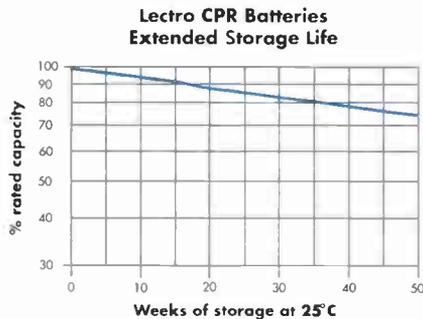
Shelf life for the Lectro CPR Battery is substantially longer than conventional lead-calcium CATV batteries. In actual tests, our batteries retained more than 70% of initial charge after being stored for one year. Typically, conventional CATV batteries require a "refresher charge" every 6 months in order to maintain peak performance.
