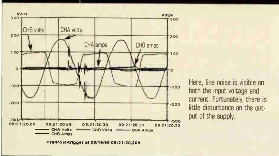
problem for a nonstandby power supply. A UPS with batteries will simply "ride through" the event on its batteries and resume drawing utility power when AC input returns. The network never sees an interruption.
