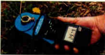
LEM Instrument's GEO Model 15 is a battery-operated, auto-ranging, ground-resistance tester with a beeper that allows one-handed checking of ground grid connections without the need for stakes or disconnections. Model 15 measures from 0.025 ohms to 1,500 ohms at 1.667 kHz and can measure leakage currents down to 1  $\mu$ A resolution. The tester comes with battery, heavy-duty case and calibration loop.
