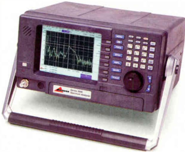
**The instrument of choice for analyzing ingress problems is a spectrum analyzer because of its broad input, excellent resolution, wide dynamic range and high sensitivity.**
