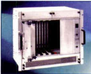
for CompactPCI. The enclosure features a plug-in power supply combination to be used in a high availability environment where withstanding excessive shock and vibration is critical. Reverse impeller-style fan modules are located in the top of the unit. The two pluggable modules are accessible from the front and can be removed for repair or maintenance. A microcontroller based on the Ultra-Smart Module option monitors voltage and temperature and controls fan speed.
