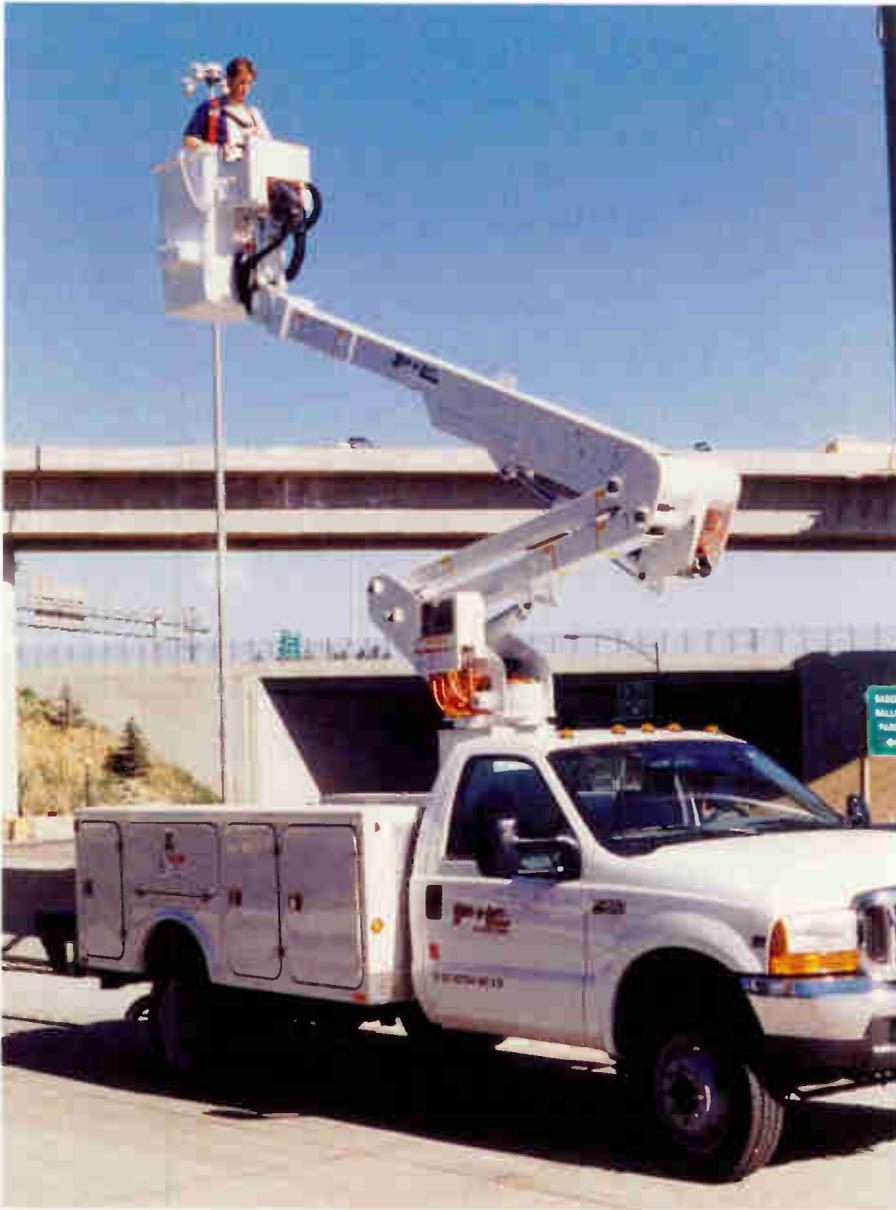
Though it looks simple, working with bucket trucks carries numerous risks, from getting “bounced” out of the bucket by an impact with another vehicle to ripping down a restaurant’s drive-through awning.
