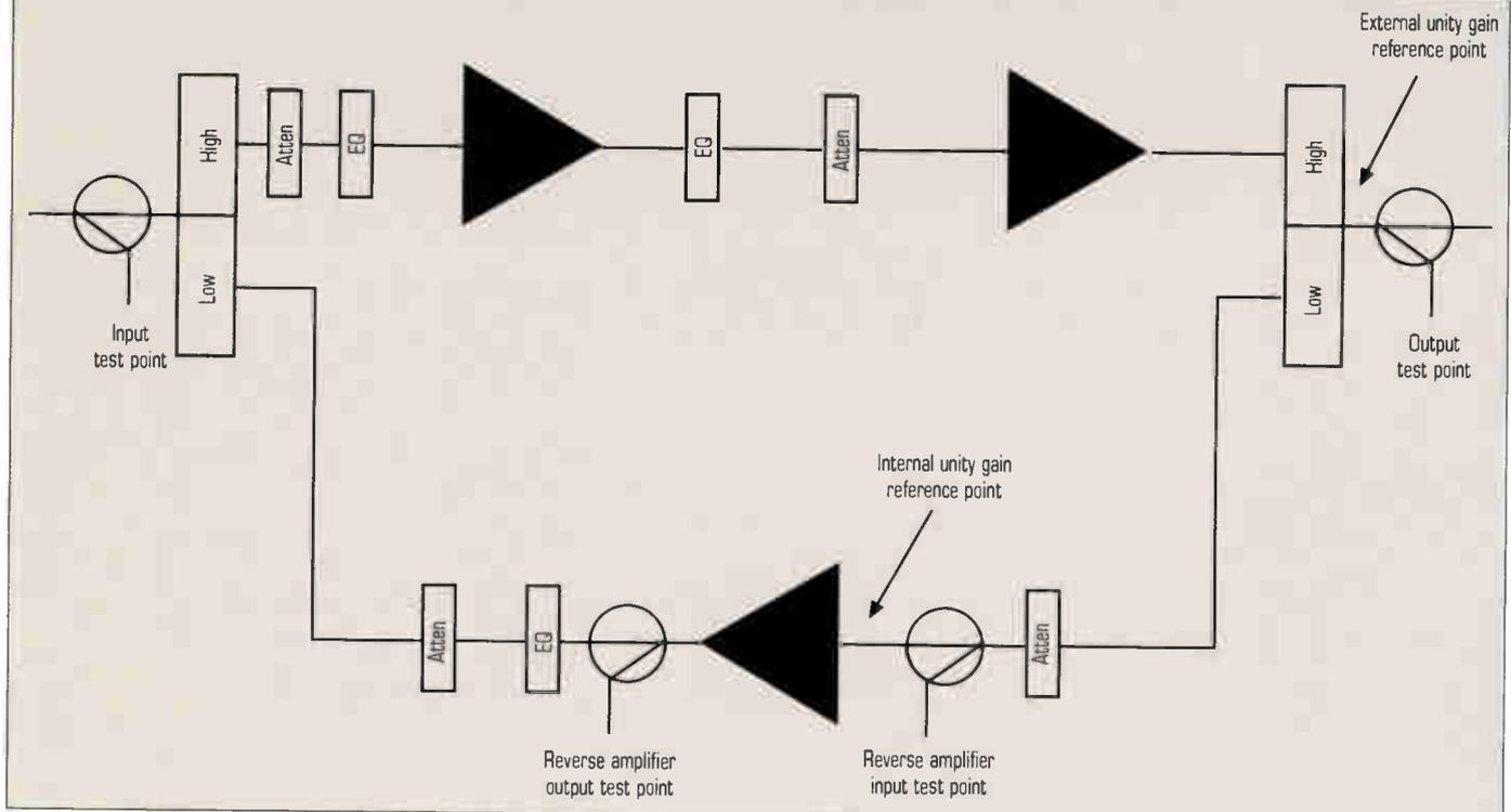
directional coupler's tap leg to the diplex filter and through the low-pass section of the diplex filter to the input of the reverse amp.
