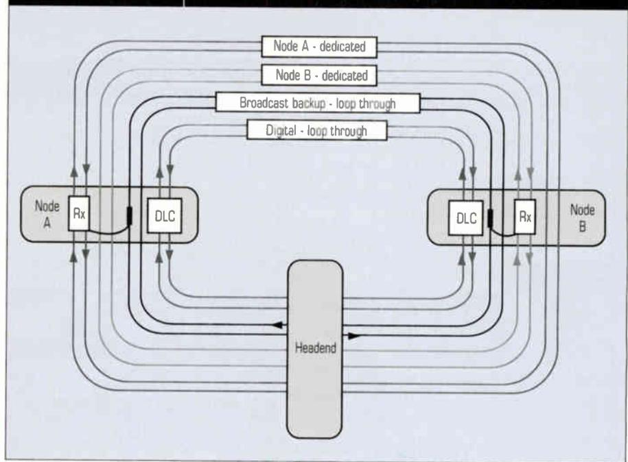
"ring-in-ring" architecture while building the network. (See Figure 1.) The style was deployed specifically for telephony because it adds a layer of redundancy, which is vital for reliability in critical communications applications such as lifeline telephony. Simply put, the design calls for dual routes to each fiber node. The nodes are outfitted with duplicate transmitters and receivers and an RF switch. (See Figure 2.)
