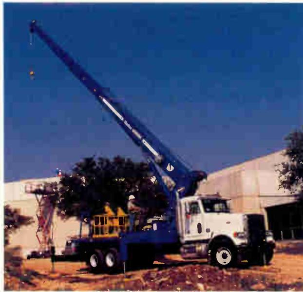
Large vehicles such as this truck-mounted crane underscore the need for well-trained drivers. Backing such a rig should be avoided if possible, but a skilled driver should be able to do so safely if necessary.
