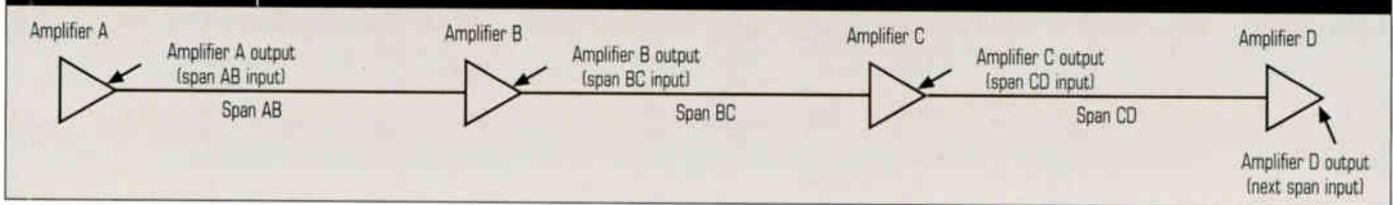
equal to the total loss of the cable and passive devices immediately upstream from that amplifier. This concept is known as unity gain, and is still a critical parameter in modern cable system design and operation.
