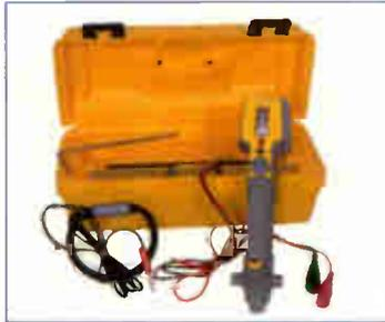
nection, coupler induction and transmitter induction. By attaching to an optional ground return probe, the 8858 becomes a fault-locating unit.
