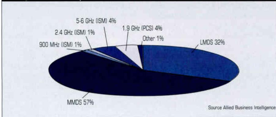
But the higher the frequency, the less likely it is for carriers to put their spectrum to use for business customers. The reason is scope of reach: LMDS and higher frequencies have a more limited range than MMDS. LMDS, for example, has a radio range of two to three miles, while MMDS has a 25- to 30-mile radius.
