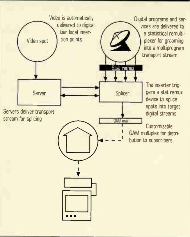
a TSI ad inserter can be connected, and the system is up and running in less than five rack units of space.
