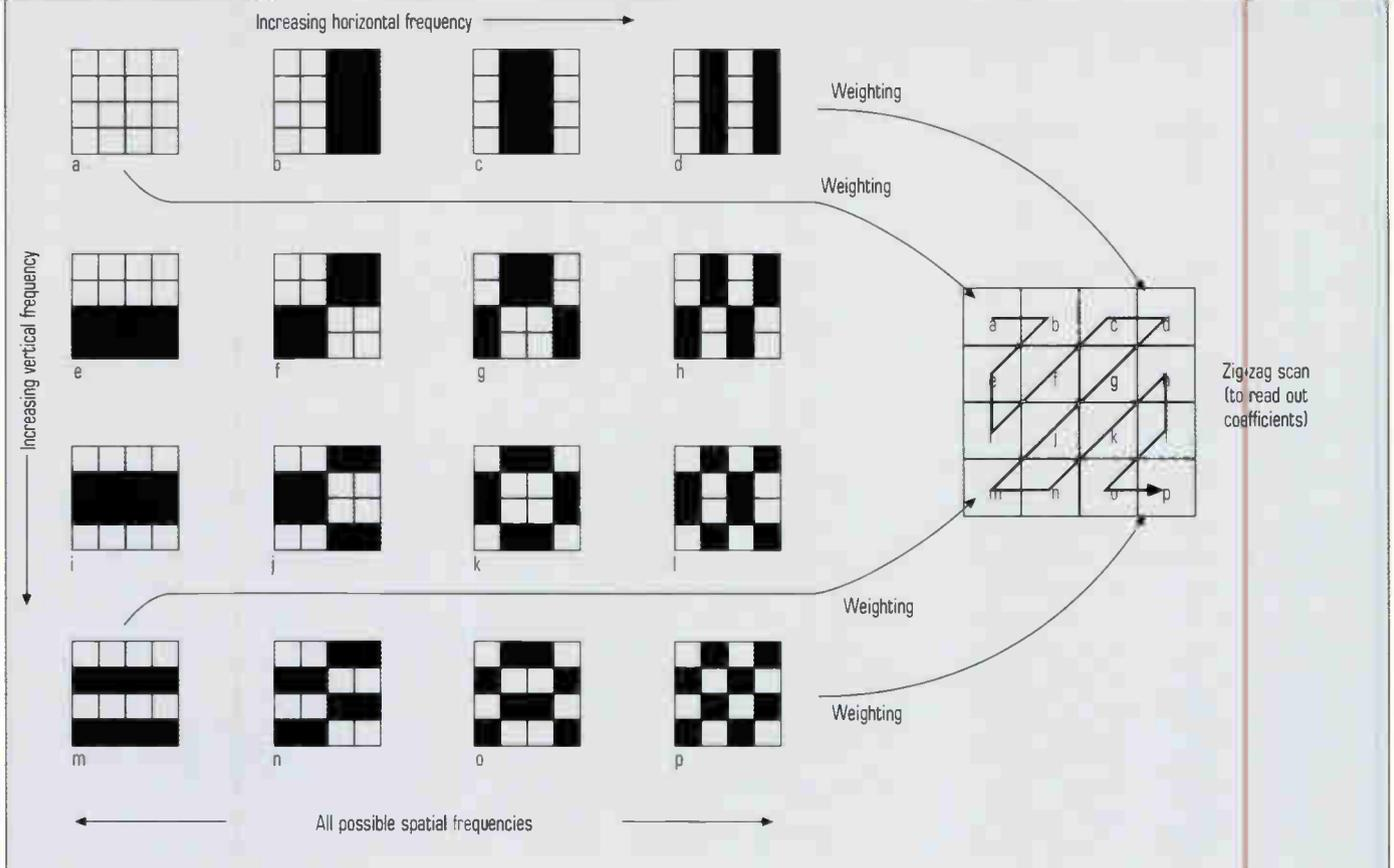
would figure out what the average value of the video is in the real picture block and assign the appropriate weighting factor to block A. This weighting goes in the DCT block shown at the right of Figure 2, at location A. This DCT block is nothing more than a way to keep track of the appropriate weightings for each of the 16 patterns in the left part of Figure 2. Just so you know, in the real world of Moving Picture Experts Group (MPEG) compression, the block is 8 x 8 and has 64 unique patterns.
