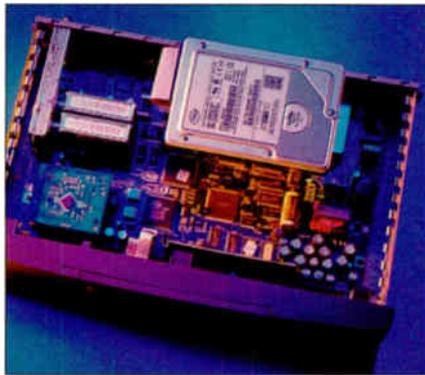
video stream and local storage in the set-top box to allow creative enhancements to content, such as highlights, interactivity and intelligent recording. The XTV Pace set-top box includes a 20 GB hard disk, allowing the device
