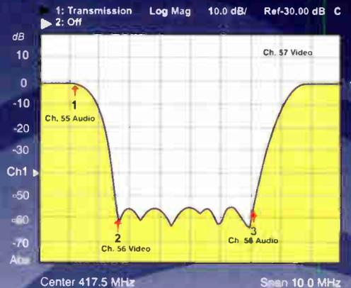
**The CD-9002 will delete an entire television or LAN channel and allow a new television channel or data to be reinserted.**
