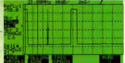
Fast Zero Span Mode for accurate measurement of return path modem signals.
