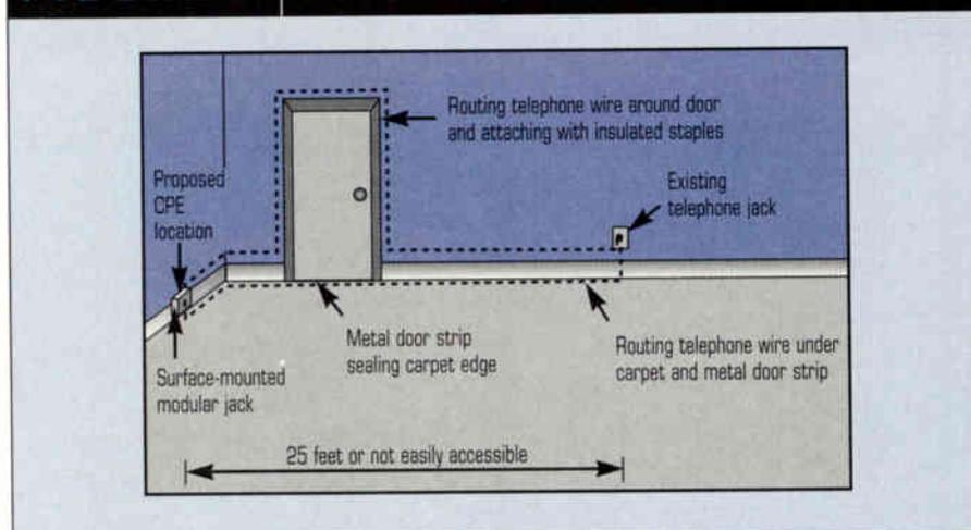
**FIGURE 2** EXTENDING AND CONVERTING A SINGLE PHONE OUTLET INTO A DOUBLE OUTLET.
