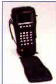
choice of viewing individual channel power readings or single, multiple or an all-channel spectrum. Automatic calibration corrects variations due to frequency response, temperature changes, and internal attenuator settings. An FM demodulator provides audio output.
