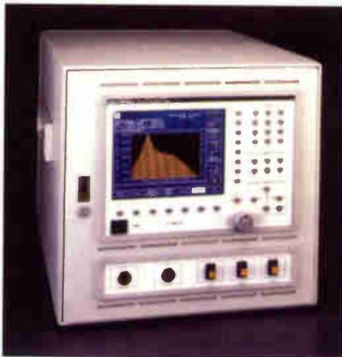
(WDM) component, amplifier and system testing. The SSB-9200 can accommodate up to 48 individual distributed feedback (DFB) laser sources for high-channel count systems.
