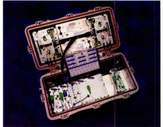
Harmonic's NODEcmts: a bi-directional optical transmission technology
